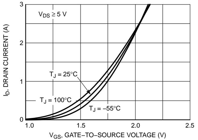
Figure 2. Transfer Characteristics
