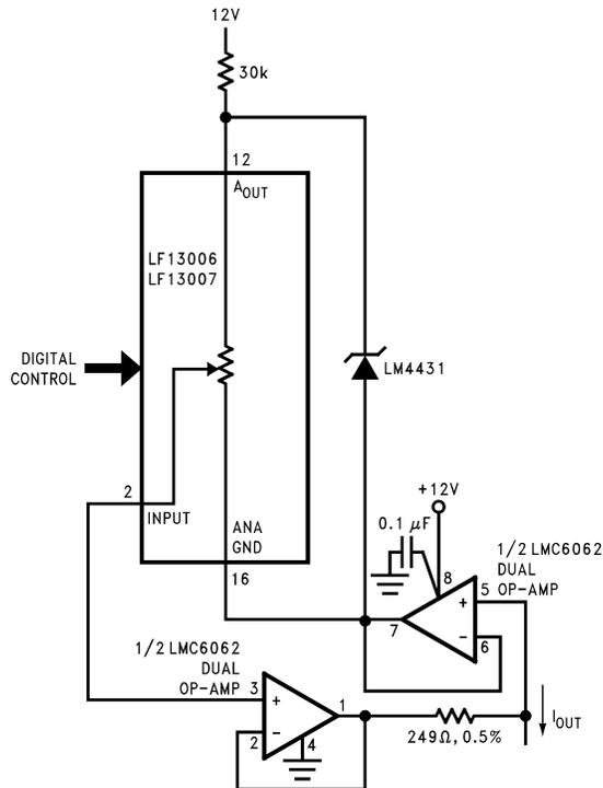
$$I_{OUT} = \frac{2.5V}{249\Omega} \left[ \frac{1}{\text{gain set \#}} \right]$$
