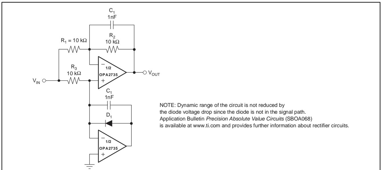
Figure 8. Precision Full-Wave Rectifier with Full Dynamic Range
