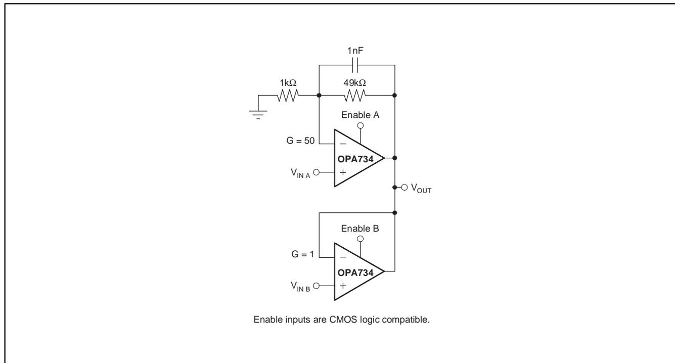
Figure 9. High-Precision 2-Input MUX for Programmable Gain
