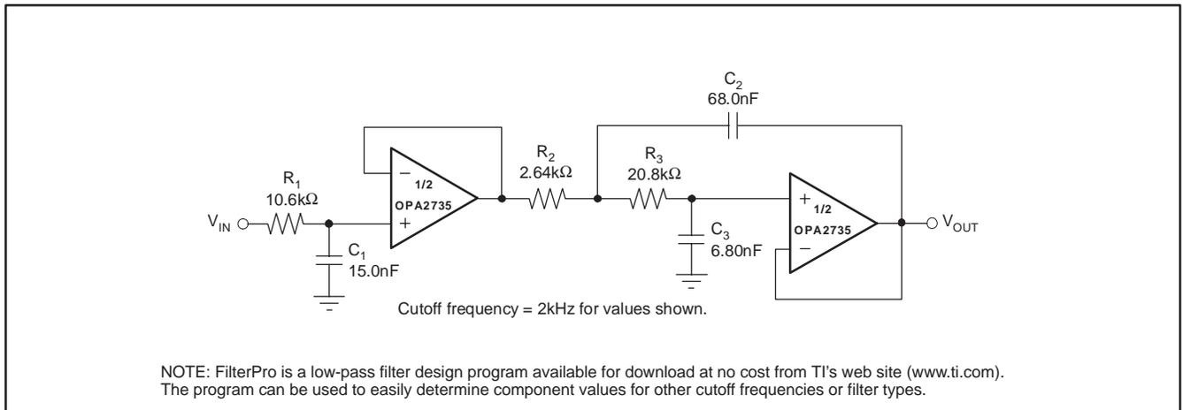
Figure 7. High DC Accuracy, 3-Pole Low-Pass Filter
