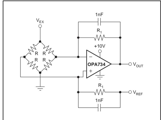
**Figure 2. Single Op Amp Bridge Amplifier Circuit**
