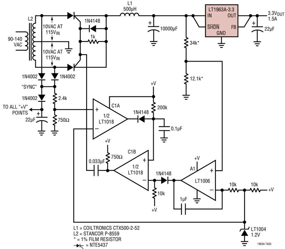
Paralleling of Regulators for Higher Output Current
