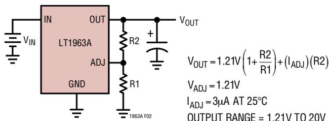
Figure 2. Adjustable Operation
