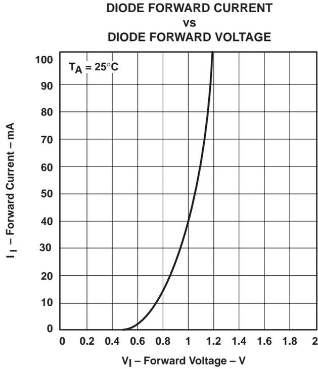
Figure 4. Typical Input Current vs Input Voltage
