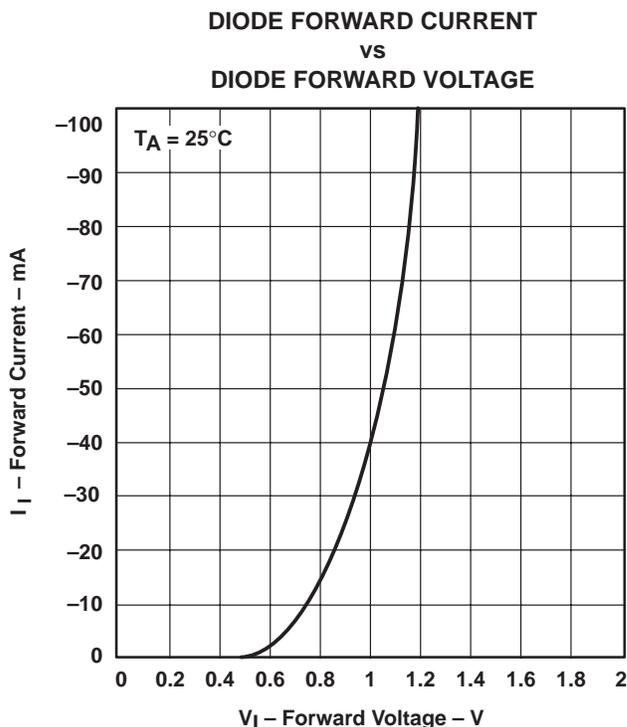
Figure 3. Typical Input Current vs Input Voltage
