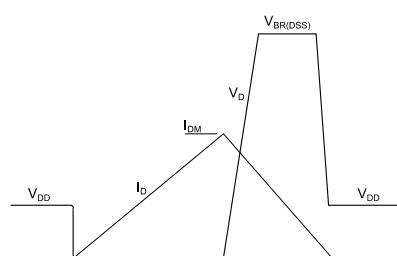
**Figure 18: Switching time waveform**
