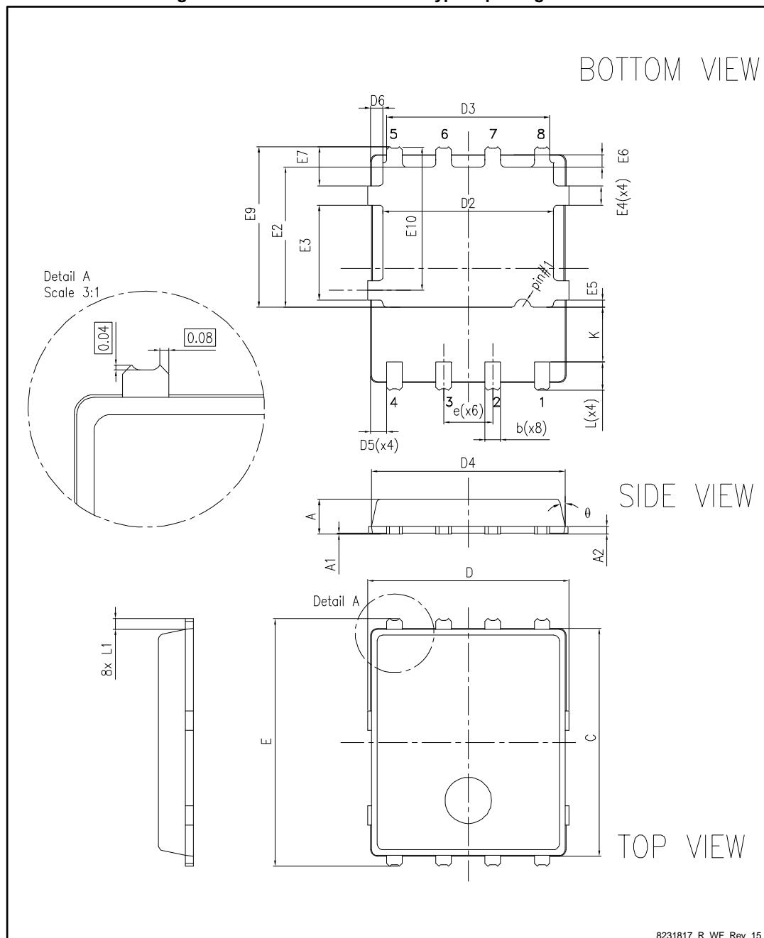
Table 8: PowerFLAT™ 5x6 WF type R mechanical data
