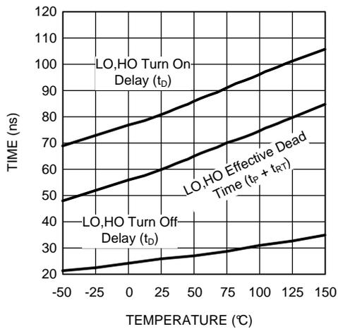
**Figure 13. Timing vs Temperature RT = 10K**
