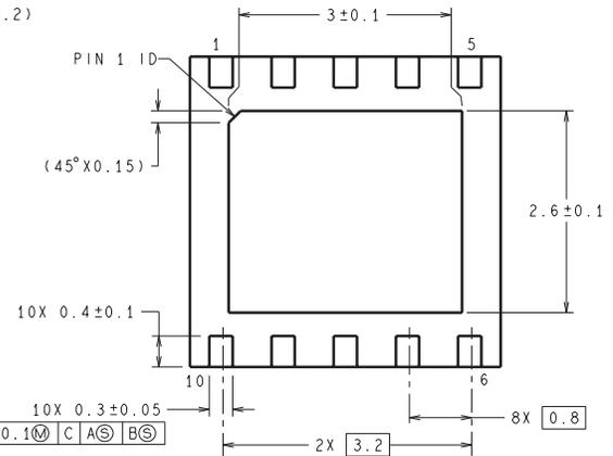
DIMENSIONS ARE IN MILLIMETERS
