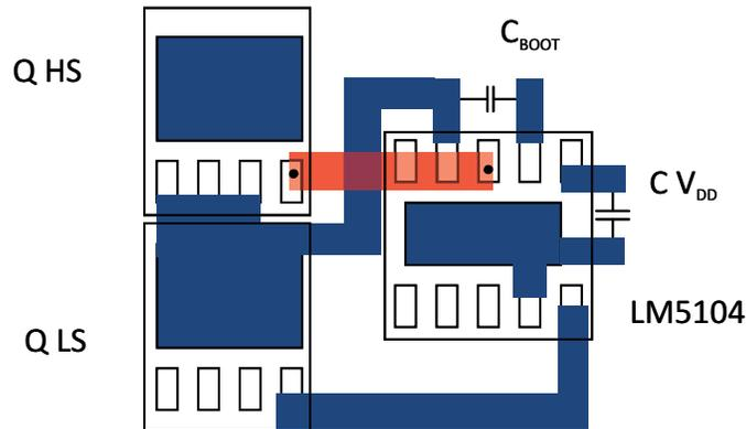
**Figure 21. LM5104 Component Placement**
