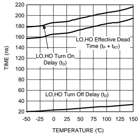
**Figure 14. Timing vs Temperature RT = 100K**
