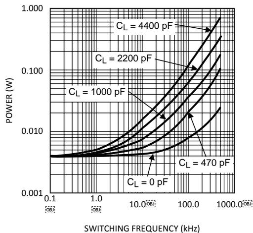
**Figure 18. Gate Driver Power Dissipation (LO + HO)
