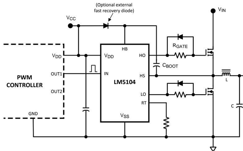
Figure 15. LM5104 Driving MOSFETs Connected in Synchronous Buck Configuration
