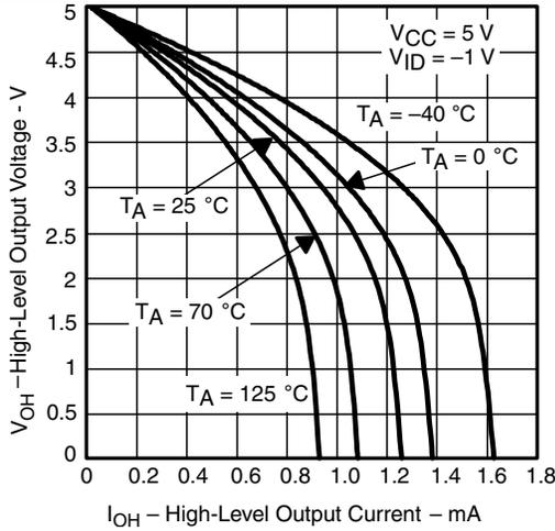
Figure 5. High-Level Output Voltage vs High-Level Output Current
