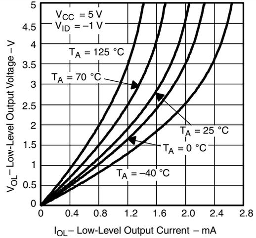
Figure 6. Low-Level Output Voltage vs Low-Level Output Current
