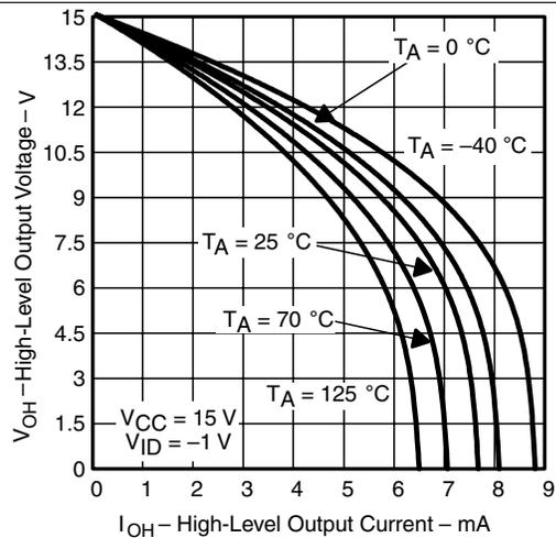
Figure 7. High-Level Output Voltage vs High-Level Output Current
