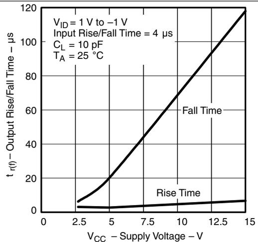
Figure 10. Output Rise/Fall Time vs Supply Voltage
