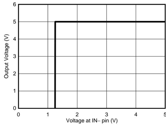
**Figure 19. Transfer Function for the Threshold Detector**
