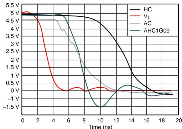
$V_{CC} = 5\text{ V}$ , Load =  $50\ \Omega / 50\text{ pF}$
