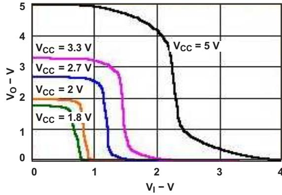
Figure 7.  $V_O$  vs  $V_I$  Characteristics of Oscillator Amplifier
