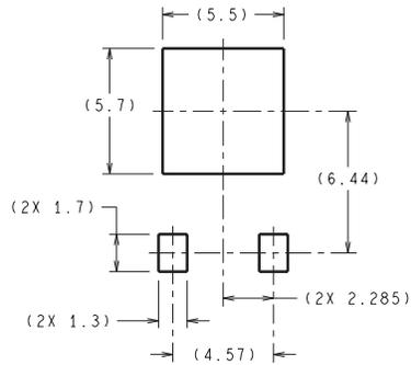
DIMENSIONS ARE IN MILLIMETERS
