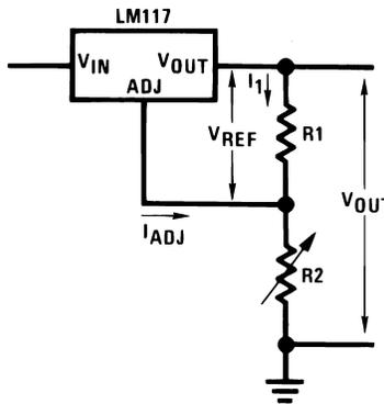
Since the 100μA current from the adjustment terminal represents an error term, the LM117 was designed to minimize  $I_{ADJ}$  and make it very constant with line and load changes. To do this, all quiescent operating current is returned to the output establishing a minimum load current requirement. If there is insufficient load on the output, the output will rise.
