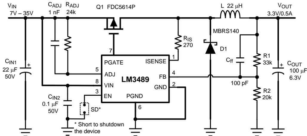
Figure 30. Typical Application Schematic for V<sub>OUT</sub> = 3.3V/500mA
