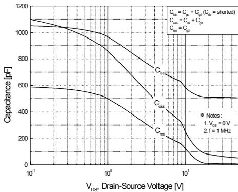
**Figure 5. Capacitance Characteristics**
