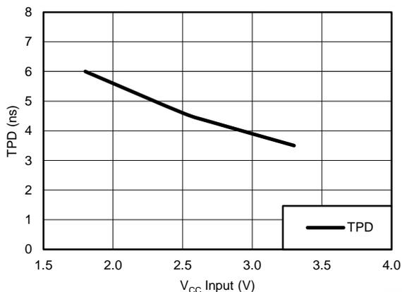
Figure 1. TPD vs V<sub>CC</sub> (T<sub>A</sub> = 25°C)
