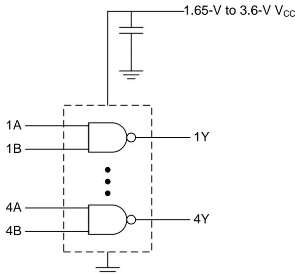
**Figure 3. Typical NAND Gate Application and Supply Voltage**
