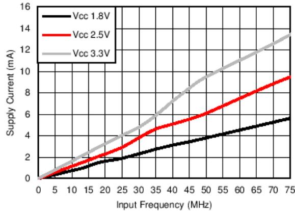
Figure 4. I<sub>CC</sub> vs Frequency
