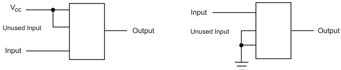
Figure 5. Layout Diagram
