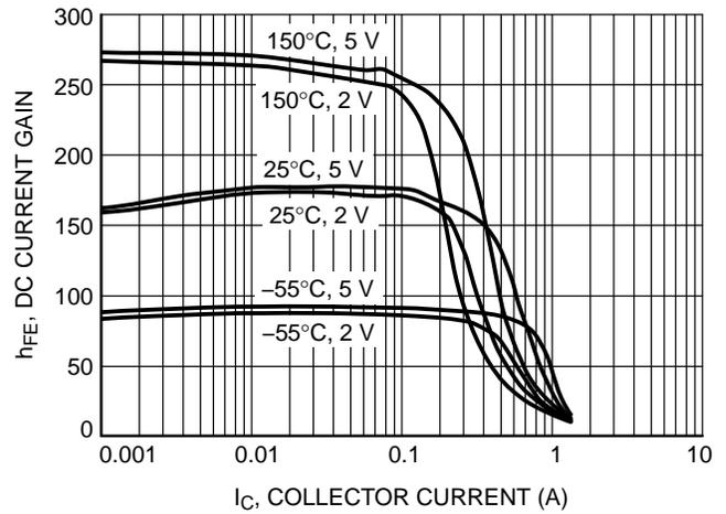
**Figure 4. DC Current Gain vs. Collector Current (BCP53-16)**
