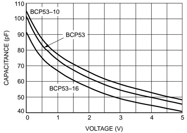
**Figure 10. Input Capacitance**
