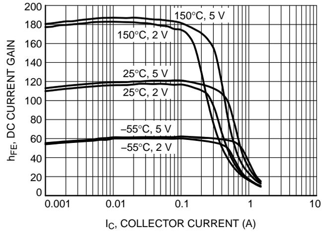
**Figure 2. DC Current Gain vs. Collector Current (BCP53)**
