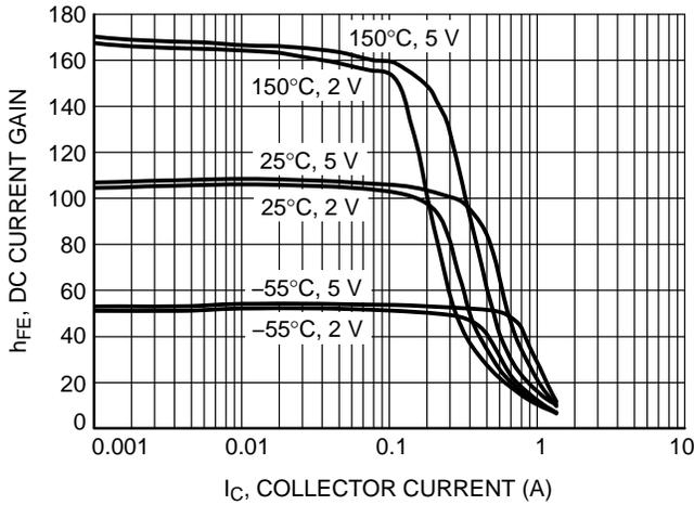
**Figure 3. DC Current Gain vs. Collector Current (BCP53-10)**
