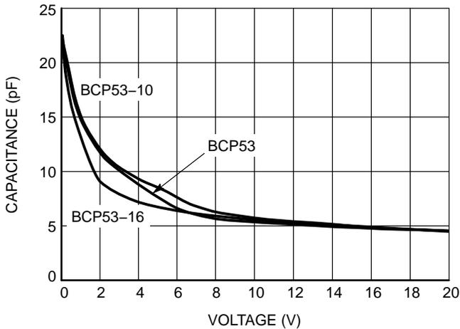
**Figure 11. Output Capacitance**
