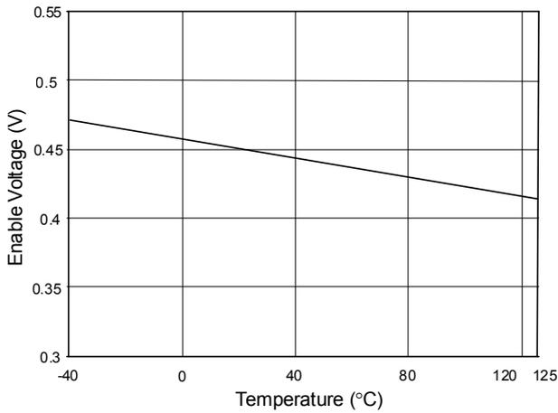
Fig. 7 Enable Voltage vs. Temperature
