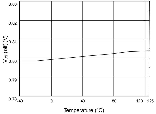
Fig. 8 V<sub>CS</sub> (off) vs. Temperature
