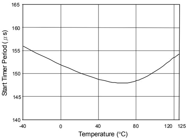
Fig. 11 Start Timer Period vs. Temperature
