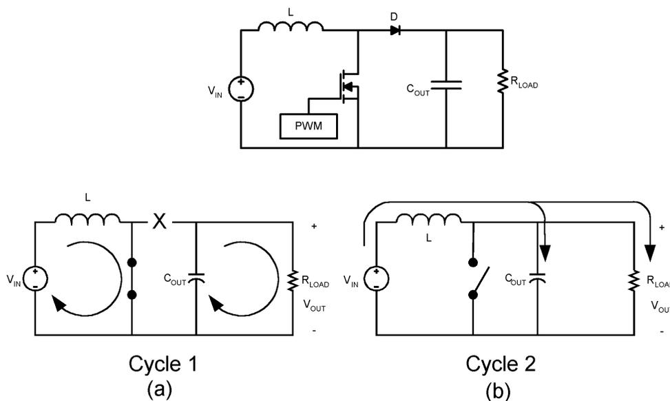
**Figure 21. Simplified Boost Converter Diagram**
