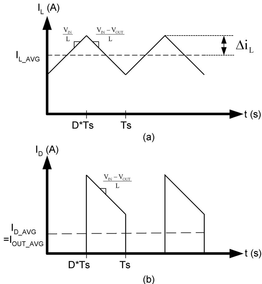
Figure 22. (a) Inductor current. (b) Diode current.
