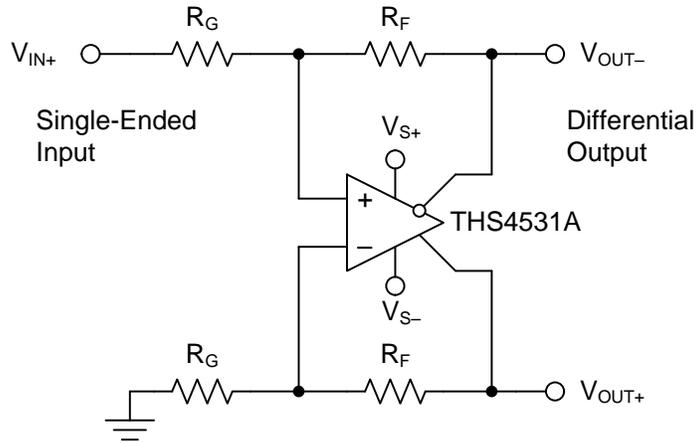
**Figure 95. Single-Ended Input to Differential Output Amplifier**
