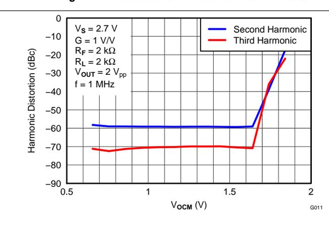
Figure 12. Harmonic Distortion vs  $V_{OCM}$  at 1 MHz
