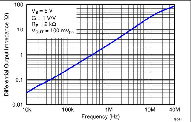
Figure 49. Main Amplifier Differential Output Impedance vs Frequency
