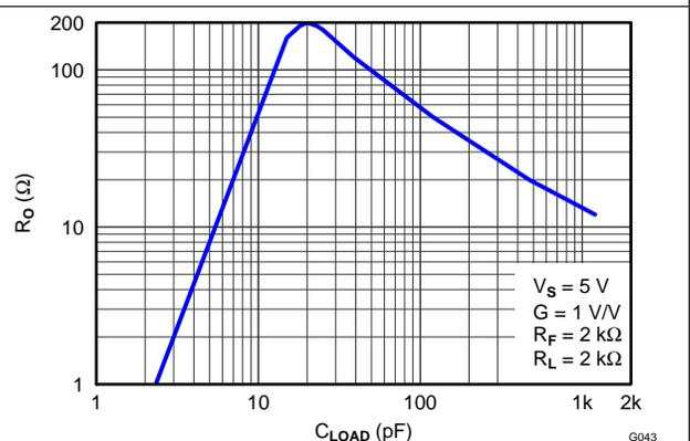
Figure 51.  $R_O$  vs  $C_{LOAD}$
