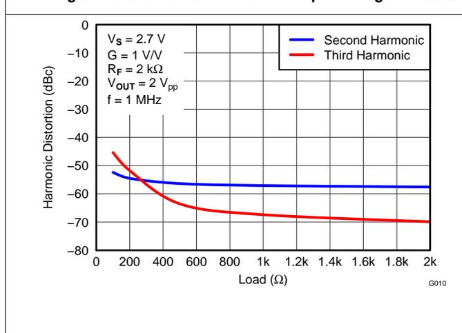
Figure 11. Harmonic Distortion vs Load at 1 MHz
