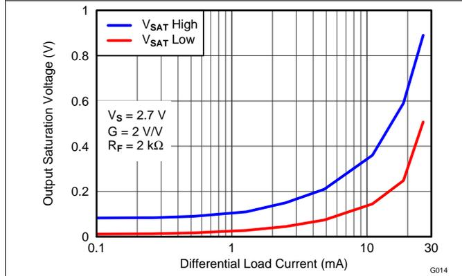
Figure 15. Single-Ended Output Saturation Voltage vs Load Current
