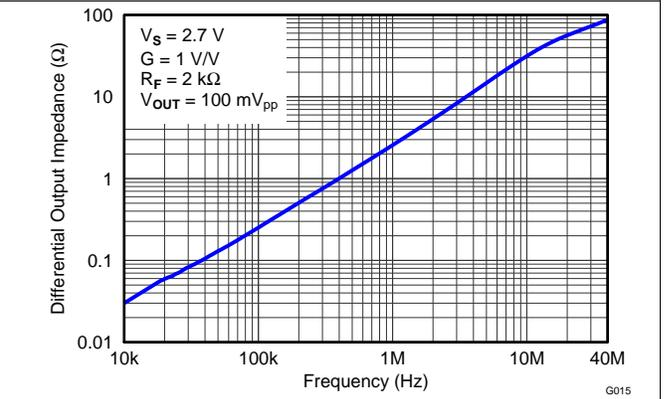
Figure 16. Main Amplifier Differential Output Impedance vs Frequency
