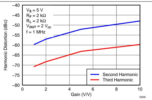
Figure 43. Harmonic Distortion vs Gain at 1 MHz
