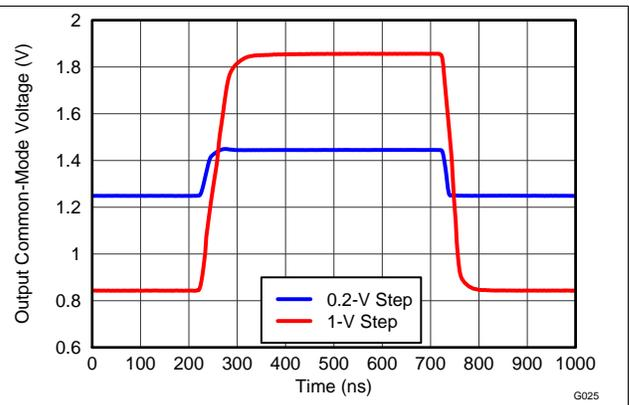
Figure 26.  $V_{OCM}$  Large- and Small Signal Pulse Response
