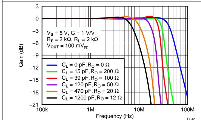
Figure 50. Frequency Response vs  $C_{LOAD}$
