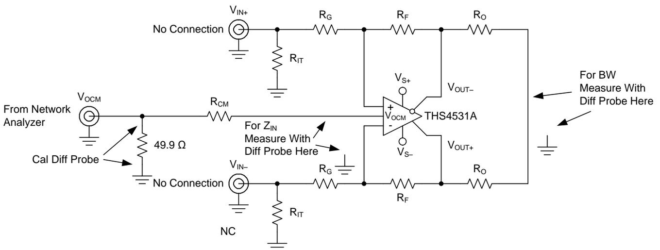
Figure 74. V<sub>OCM</sub> Input Test Circuit
