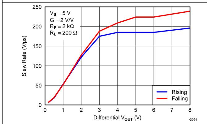
**Figure 38. Differential Slew Rate vs  $V_{OUT}$  Step**
