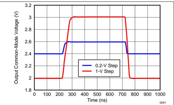
Figure 59.  $V_{OCM}$  Large- and Small Signal Pulse Response
