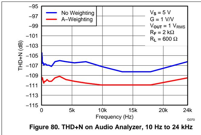
Figure 80. THD+N on Audio Analyzer, 10 Hz to 24 kHz
