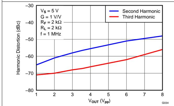
Figure 42. Harmonic Distortion vs Output Voltage at 1 MHz
