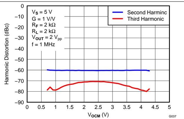
Figure 45. Harmonic Distortion vs  $V_{OCM}$  at 1 MHz
