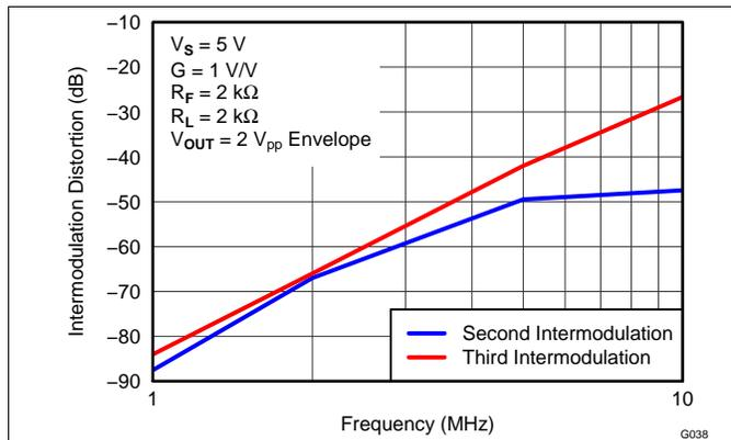
Figure 46. Two-Tone, 2<sup>nd</sup> and 3<sup>rd</sup> Order Intermodulation Distortion vs Frequency
