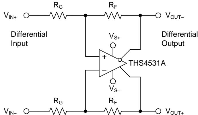
Figure 92. Differential Input to Differential Output Amplifier
