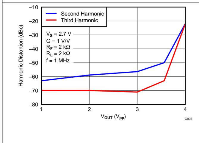
Figure 9. Harmonic Distortion vs Output Voltage at 1 MHz
