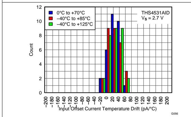
Figure 29. Input Offset Current Temp Drift Histogram
