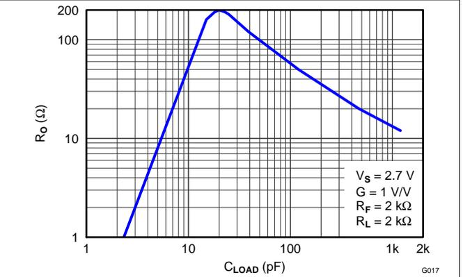
Figure 18.  $R_O$  vs  $C_{LOAD}$
