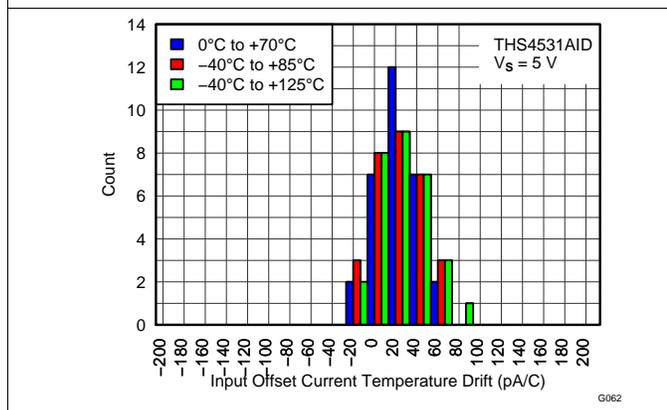
Figure 62. Input Offset Current Temp Drift Histogram
