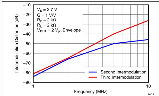
Figure 13. Two-Tone, 2<sup>nd</sup> and 3<sup>rd</sup> Order Intermodulation Distortion vs Frequency
