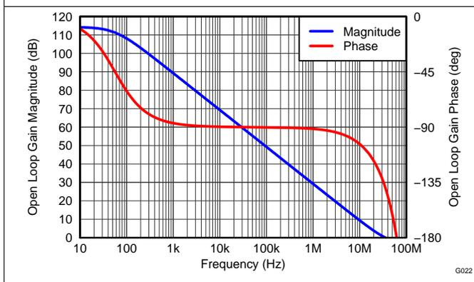
Figure 23. Main Amplifier Differential Open-Loop Gain and Phase vs Frequency
