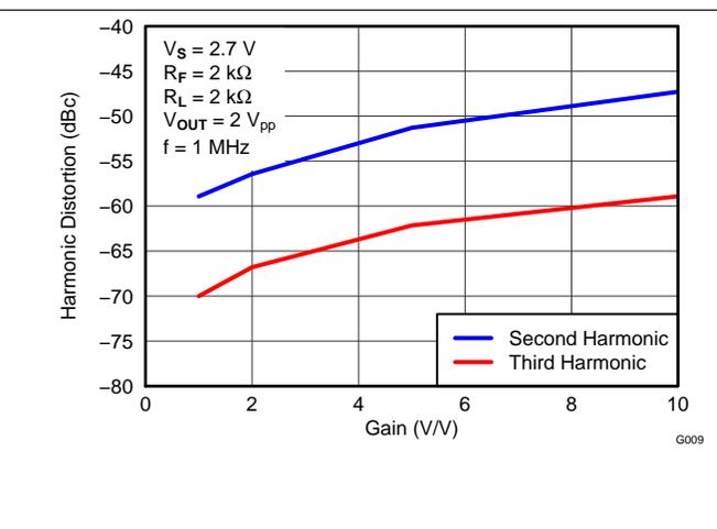
Figure 10. Harmonic Distortion vs Gain at 1 MHz
