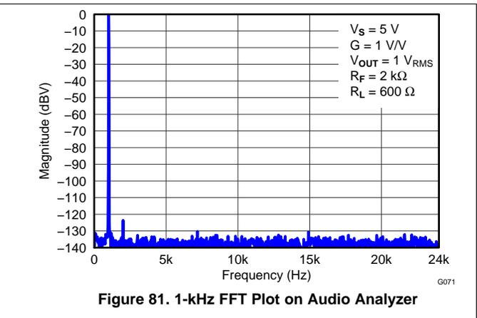
Figure 81. 1-kHz FFT Plot on Audio Analyzer
