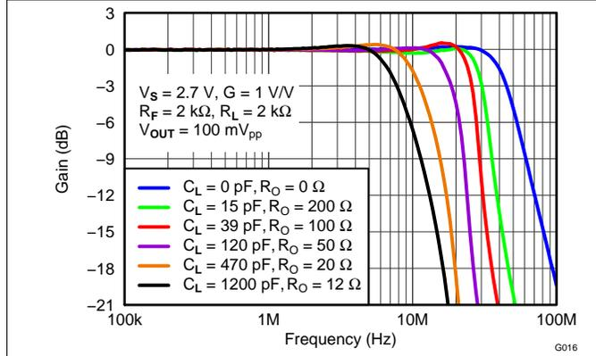
Figure 17. Frequency Response vs  $C_{LOAD}$
