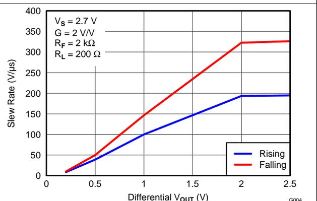
Figure 4. Single-Ended Slew Rate vs  $V_{OUT}$  Step
