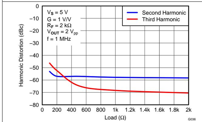
Figure 44. Harmonic Distortion vs Load at 1 MHz
