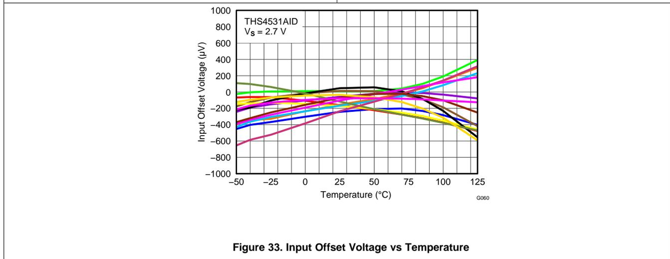
Figure 33. Input Offset Voltage vs Temperature
