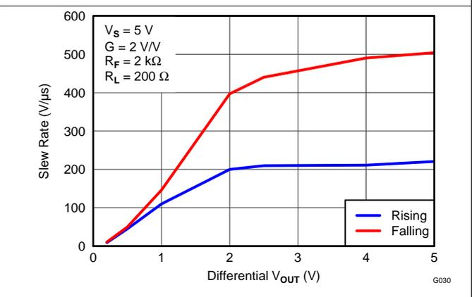
**Figure 37. Single-Ended Slew Rate vs  $V_{OUT}$  Step**
