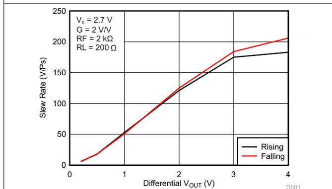
Figure 5. Differential Slew Rate vs  $V_{OUT}$  Step
