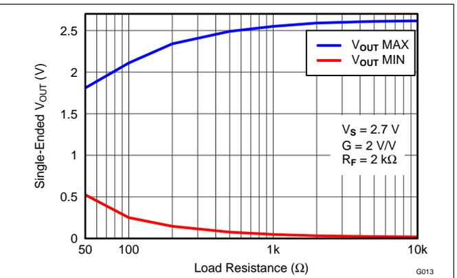
Figure 14. Single-Ended Output Voltage Swing vs Load Resistance
