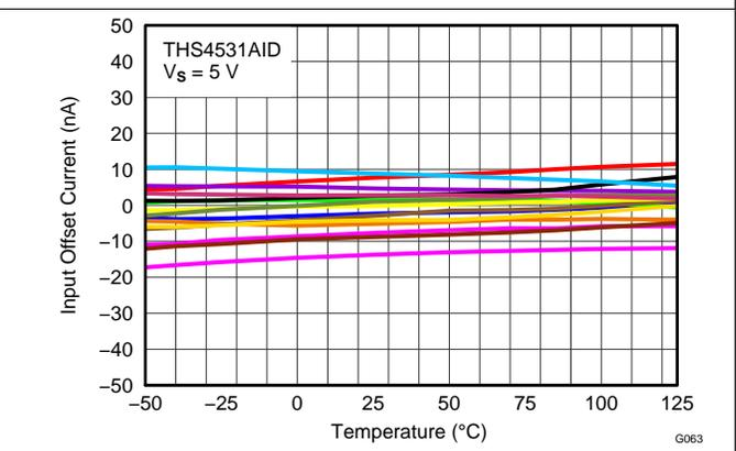
Figure 63. Input Offset Current vs Temperature
