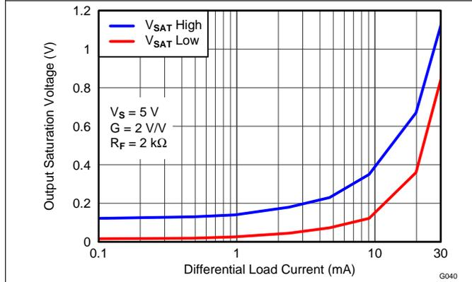
Figure 48. Single-Ended Output Saturation Voltage vs Load Current
