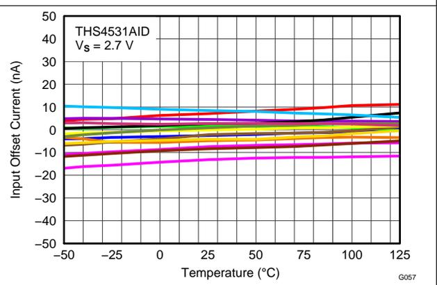
Figure 30. Input Offset Current vs Temperature
