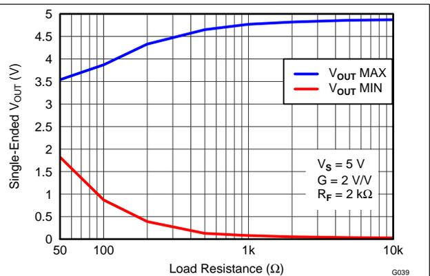
Figure 47. Single-Ended Output Voltage Swing vs Load Resistance
