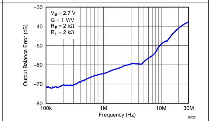
Figure 24. Output Balance Error vs Frequency
