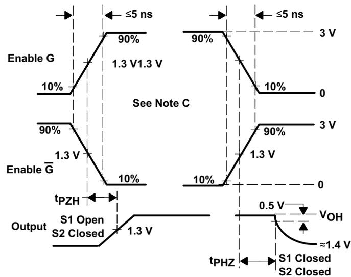
Figure 13. Voltage Waveforms For  $t_{PHZ}$ ,  $t_{PZH}$
