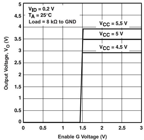
**Figure 4. Output Voltage vs Enable G Voltage**
