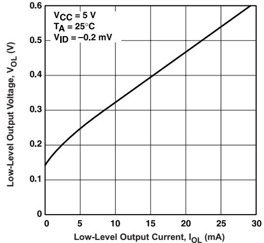
**Figure 2. Low-Level Output Voltage vs Low-Level Output Current**
