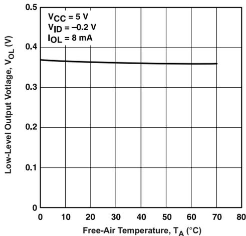
**Figure 3. Low-Level Output Voltage vs Free-Air Temperature**
