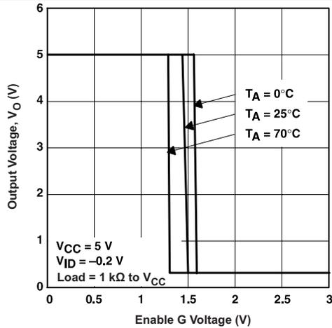
Figure 7. Output Voltage vs Enable G Voltage
