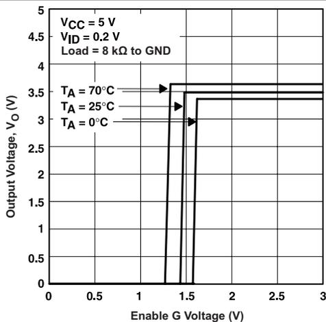
**Figure 5. Output Voltage vs Enable G Voltage**
