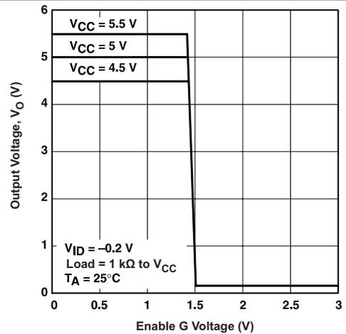
**Figure 6. Output Voltage vs Enable G Voltage**
