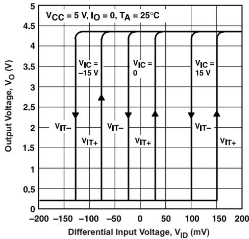
Figure 9. AM26LS33A Output Voltage vs Differential Input Voltage
