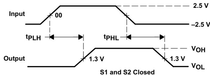
Figure 12. Voltage Waveforms For  $t_{PLH}$ ,  $t_{PHL}$
