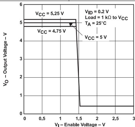
Figure 7. Output Voltage vs Enable Voltage
