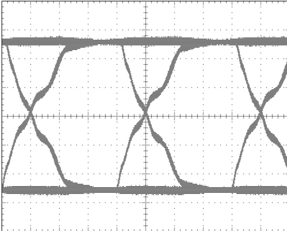
**Figure 17. Eye Diagram for 5-Mbps Over 100 feet of Standard CAT-5E cable
