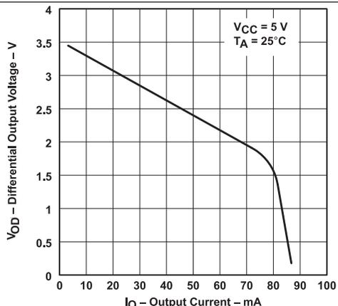
Figure 3. Driver, Differential Output Voltage vs Output Current
