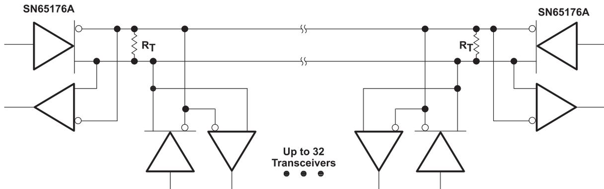
The line should be terminated at both ends in its characteristic impedance ( $R_T = Z_0$ ). Stub lengths off the main line should be kept as short as possible.
