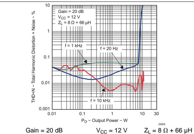
Figure 4. Total Harmonic Distortion + Noise vs Output Power
