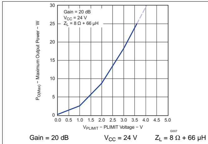
**Figure 7. Maximum Output Power vs Plimit Voltage**
