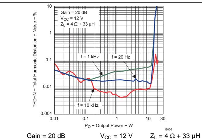
Figure 6. Total Harmonic Distortion + Noise vs Output Power
