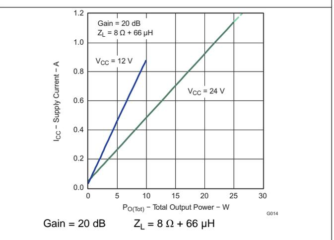
**Figure 12. Supply Current vs Total Output Power**
