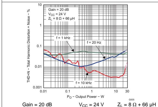
Figure 5. Total Harmonic Distortion + Noise vs Output Power
