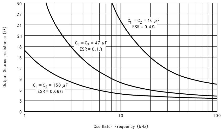
FIGURE 3. Output Source Resistance vs Oscillator Frequency
