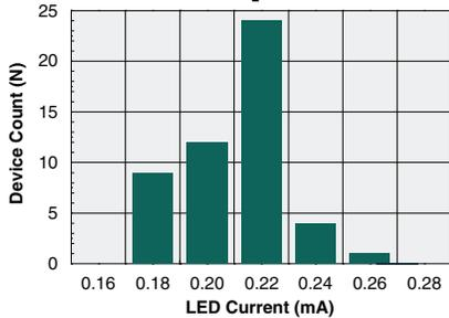
**Typical I<sub>F</sub> for Switch Dropout**
