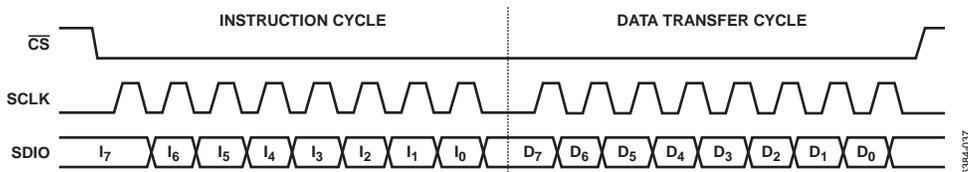
Figure 60. Serial Port Write Timing—Clock Stall Low
