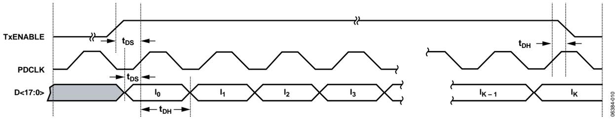
Figure 30. 18-Bit Parallel Port Timing Diagram—Interpolating DAC Mode
