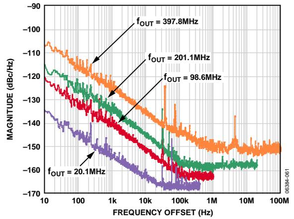
Figure 20. Residual Phase Noise, System Clock = 1 GHz
