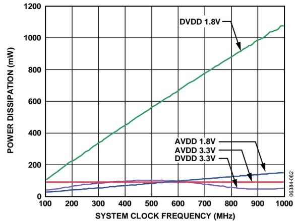
Figure 22. Power Dissipation vs. System Clock (PLL Disabled)
