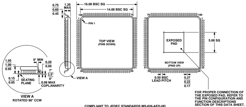
Figure 65. 100-Lead Thin Quad Flat Package, Exposed Pad [TQFP\_EP] (SV-100-4)
