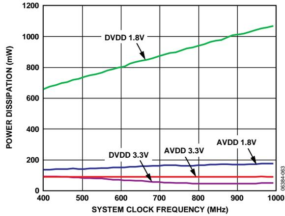
Figure 23. Power Dissipation vs. System Clock (PLL Enabled)
