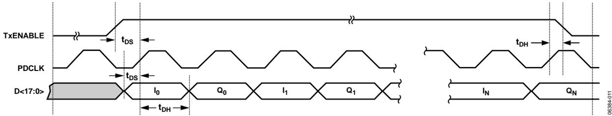
Figure 31. 18-Bit Parallel Port Timing Diagram—Quadrature Modulation Mode
