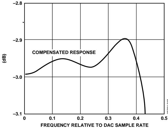
Figure 38. DAC Response with Inverse Sinc Compensation
