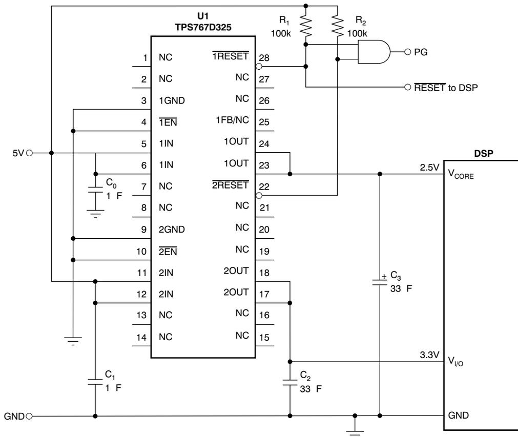
**Figure 25. Dual-Voltage DSP Application**
