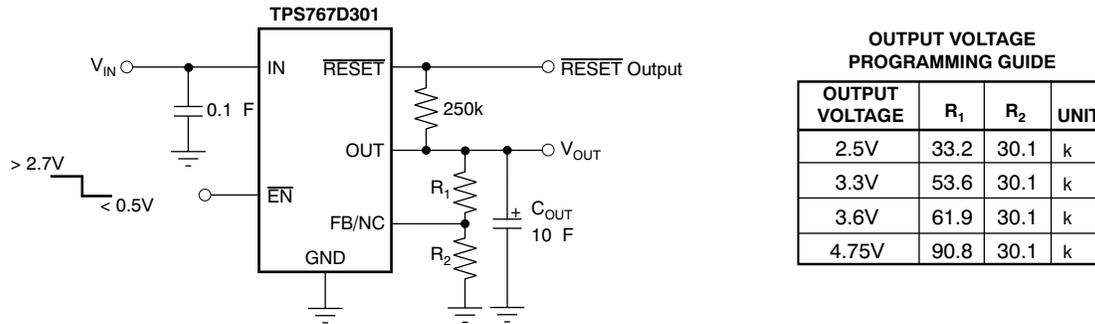
**Figure 26. TPS767D301 Adjustable LDO Regulator Programming**
