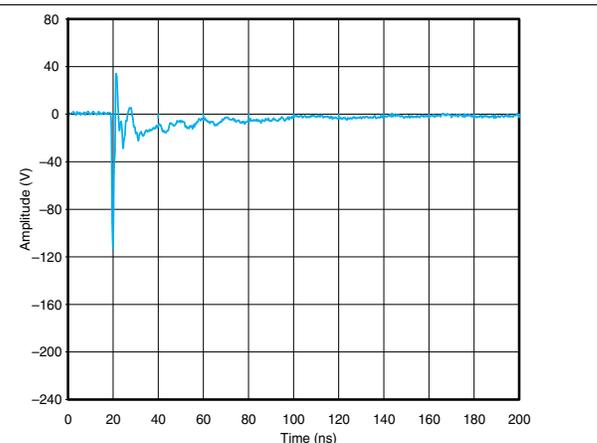
Figure 4. Figure 3. IEC Clamping Waveforms (-8-kV Contact)
