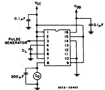
Fig. 16 - Dynamic power dissipation test circuit.
