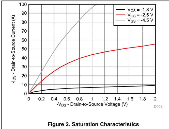
Figure 2. Saturation Characteristics
