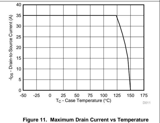
Figure 11. Maximum Drain Current vs Temperature
