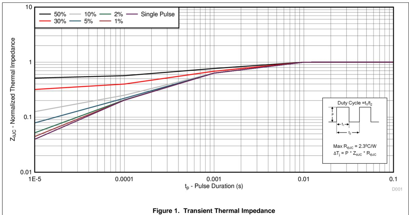
Figure 1. Transient Thermal Impedance
