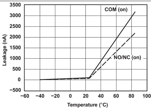
Figure 5. Leakage Current vs Temperature ( $V_{CC} = 5\text{ V}$ )
