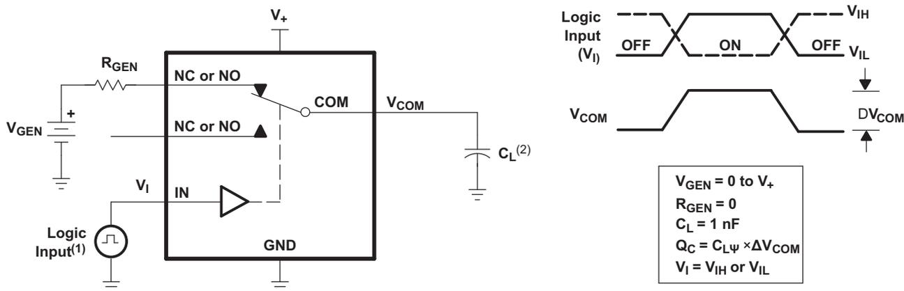
1. All input pulses are supplied by generators having the following characteristics: PRR 3 10 MHz, Z<sub>O</sub> = 50 Ω, t<sub>r</sub> < 5 ns, t<sub>f</sub> < 5 ns.
