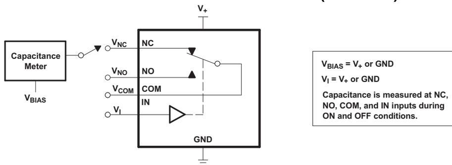
Figure 17. Capacitance ( $C_I$ ,  $C_{COM(ON)}$ ,  $C_{NC(OFF)}$ ,  $C_{NO(OFF)}$ ,  $C_{NC(ON)}$ ,  $C_{NO(ON)}$ )
