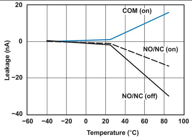
Figure 4. Leakage Current vs Temperature ( $V_{CC} = 3.3\text{ V}$ )
