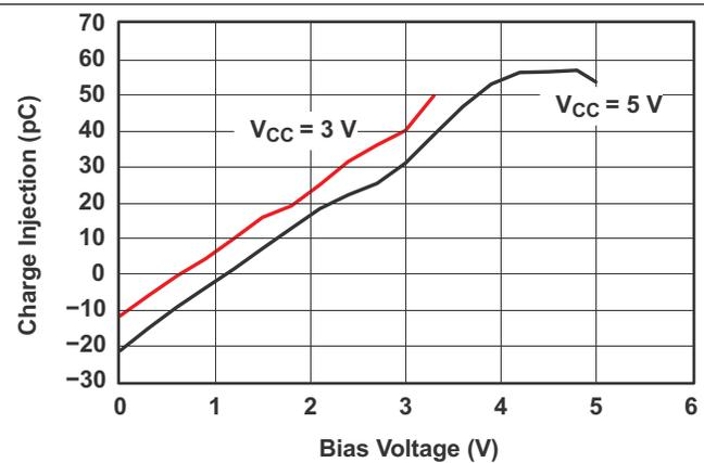
Figure 6. Charge Injection ( $Q_C$ ) vs  $V_{COM}$
