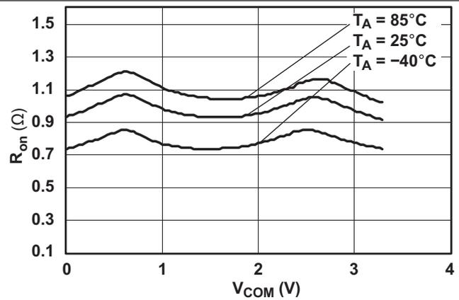
Figure 2.  $R_{on}$  vs  $V_{COM}$  ( $V_{CC} = 3.3\text{ V}$ )
