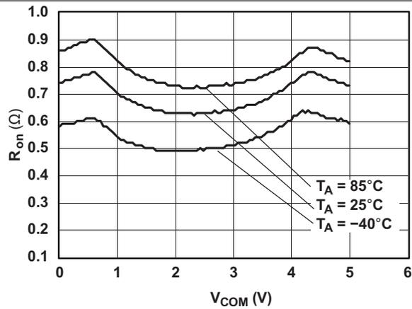
Figure 3.  $R_{on}$  vs  $V_{COM}$  ( $V_{CC} = 5\text{ V}$ )
