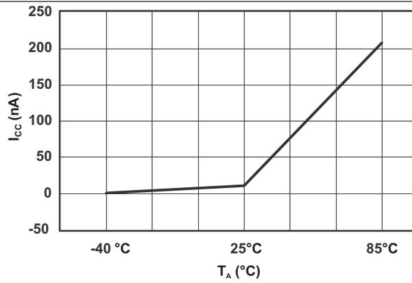
**Figure 13. Power-Supply Current vs Temperature ( $V_{CC} = 5\text{ V}$ )**
