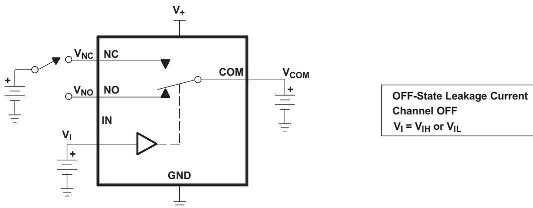
Figure 15. OFF-State Leakage Current
