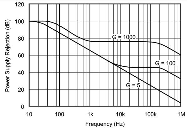
Figure 4. Negative Power Supply Rejection vs Frequency
