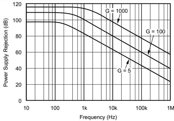
Figure 3. Positive Power Supply Rejection vs Frequency
