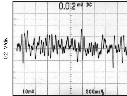
Figure 16. Voltage Noise, 0.1 Hz to 10 Hz
