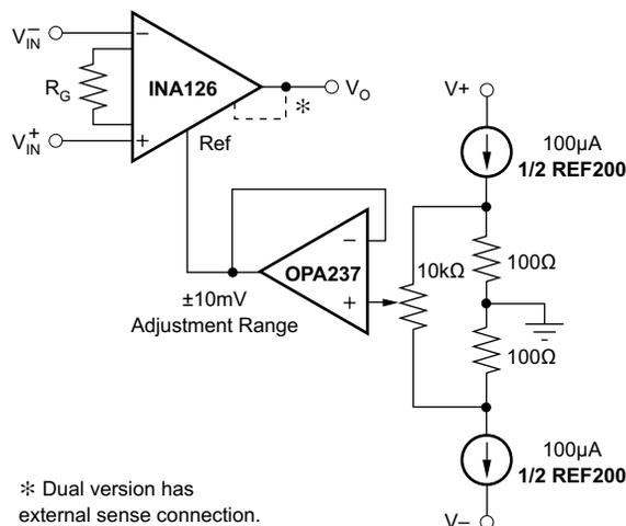
Figure 19. Optional Trimming of Output Offset Voltage
