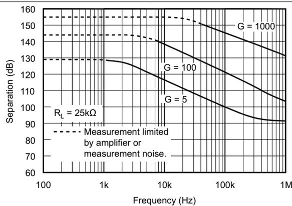
Figure 17. Channel Separation vs Frequency, RTI (Dual Version)
