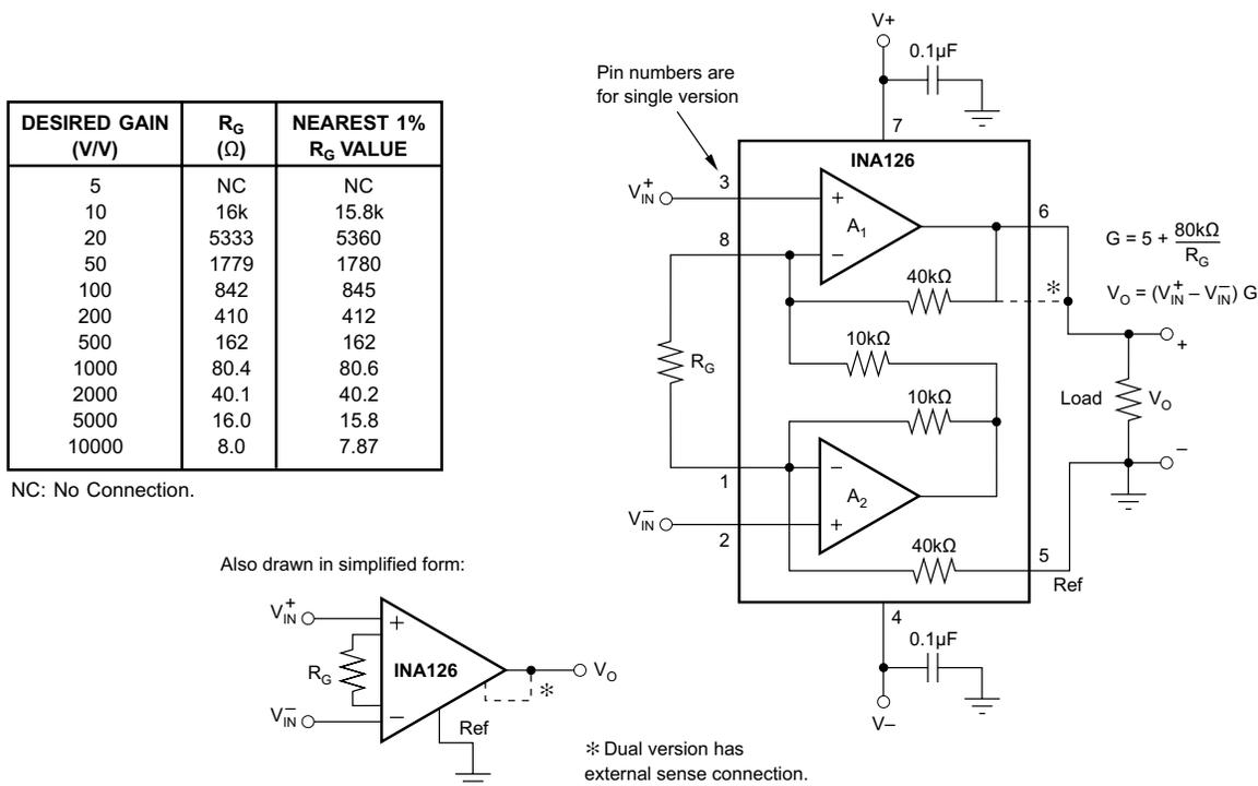
**Figure 18. Basic Connections**
