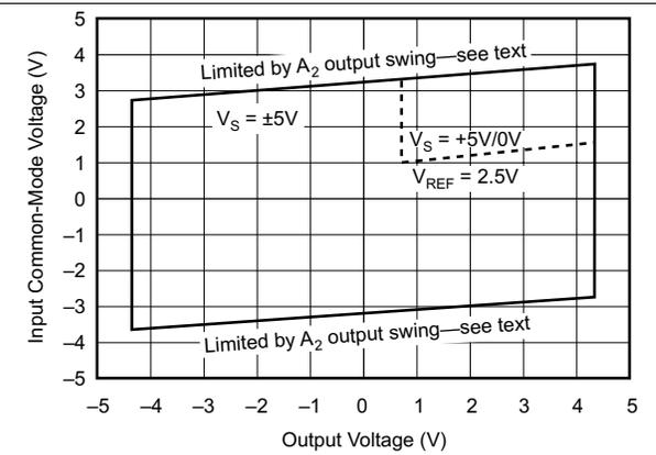
Figure 6. Input Common-Mode Voltage Range vs Output Voltage,  $V_S = \pm 5\text{ V}$
