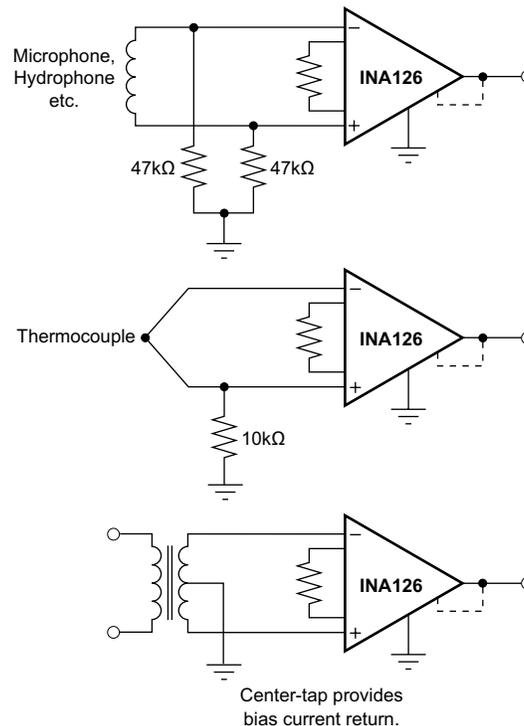
**Figure 20. Providing an Input Common-Mode Current Path**
