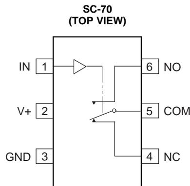
Switches are shown for logic 0 input.
