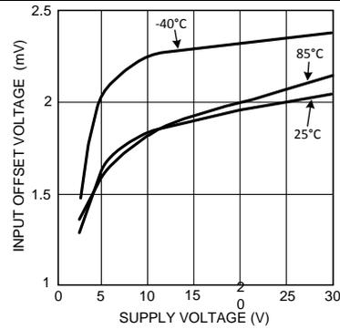
Figure 4. Input Offset Voltage vs Supply Voltage
