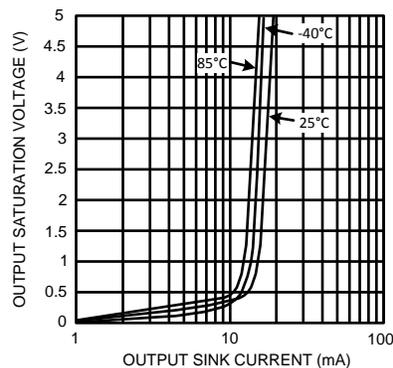
Figure 7. Output Saturation Voltage vs Output Sink Current
