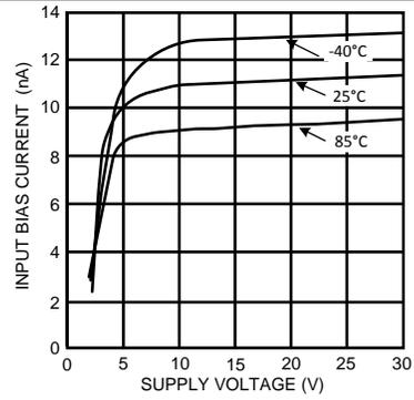
Figure 2. Input Bias Current vs Supply Current
