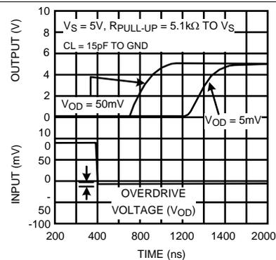
**Figure 11. Response Time for Various Input Overdrives –  $t_{PLH}$**
