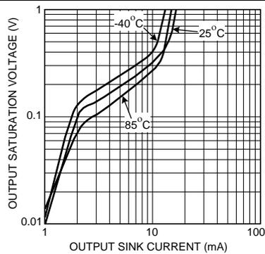
Figure 3. Output Saturation Voltage vs Output Sink Current
