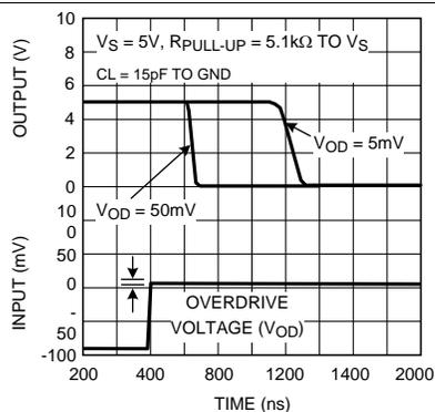
**Figure 10. Response Time for Various Input Overdrives –  $t_{PHL}$**
