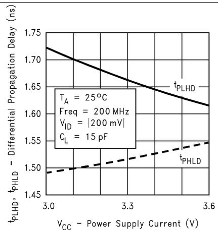
**Figure 6. Differential Propagation Delay vs Power Supply Voltage**
