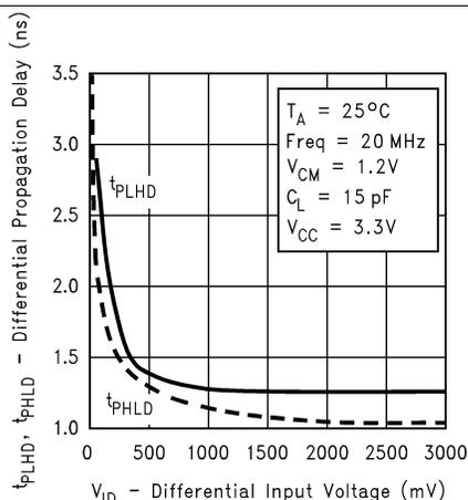
Figure 11. Differential Propagation Delay vs Differential Input Voltage
