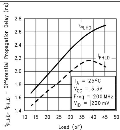
Figure 16. Differential Propagation Delay vs Load
