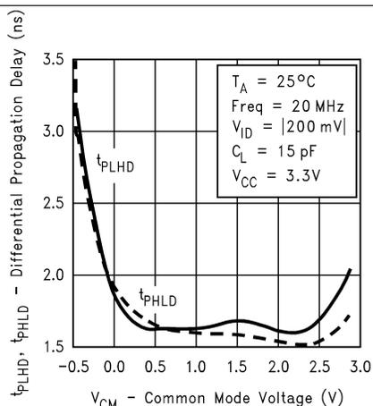
Figure 10. Differential Propagation Delay vs Common Mode Voltage
