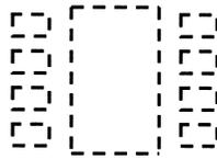
Figure 23. WSON Thermal Land Pad and Pin Pads
