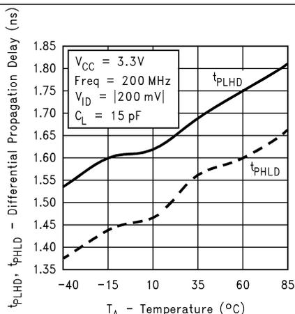
Figure 7. Differential Propagation Delay vs Ambient Temperature
