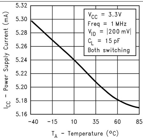
**Figure 5. Power Supply Current vs Ambient Temperature**
