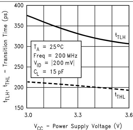
Figure 12. Transition Time vs Power Supply Voltage
