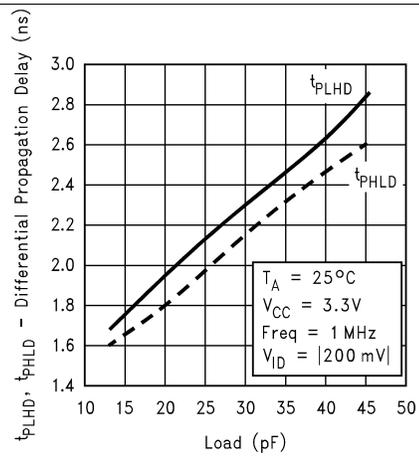
Figure 14. Differential Propagation Delay vs Load
