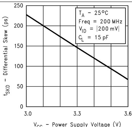
Figure 8. Differential Skew vs Power Supply Voltage
