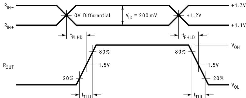
Figure 19. Receiver Propagation Delay and Transition Time Waveforms
