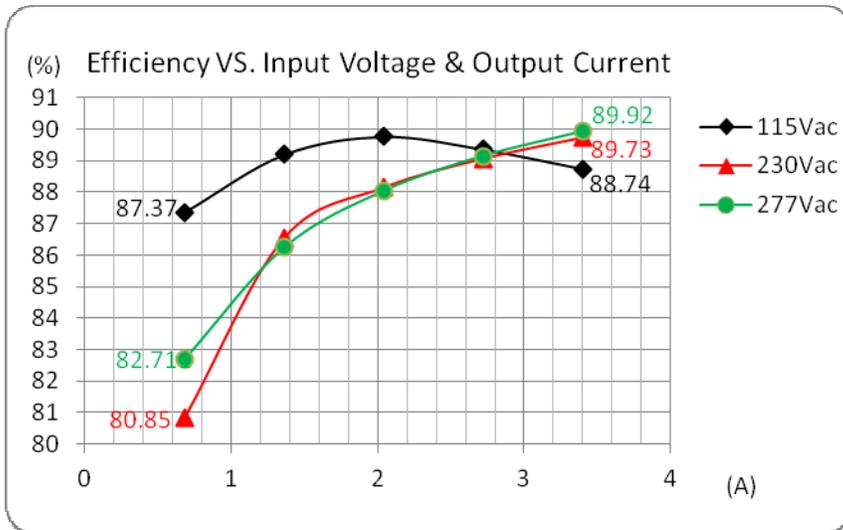
**Efficiency vs. Input Voltage and Output Current (CC Load)
