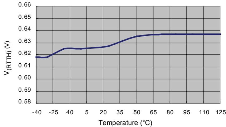
**Figure 13. Trigger Voltage for Over-Temperature Protection V<sub>RTTH</sub> vs. Temperature**
