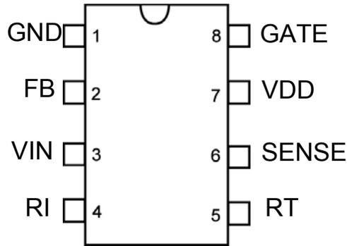
Figure 4. Pin Configuration
