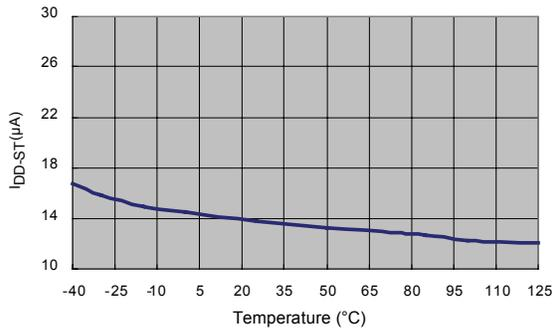
**Figure 6. Startup Current ( $I_{DD-ST}$ ) vs. Temperature**
