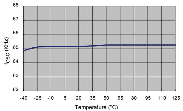
**Figure 11. PWM Frequency ( $f_{osc}$ ) vs. Temperature**
