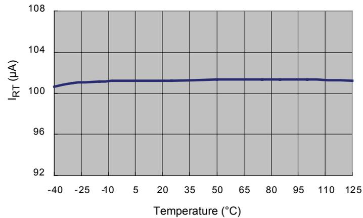
**Figure 14. Output Current of RT Pin (I<sub>RT</sub>) vs. Temperature**
