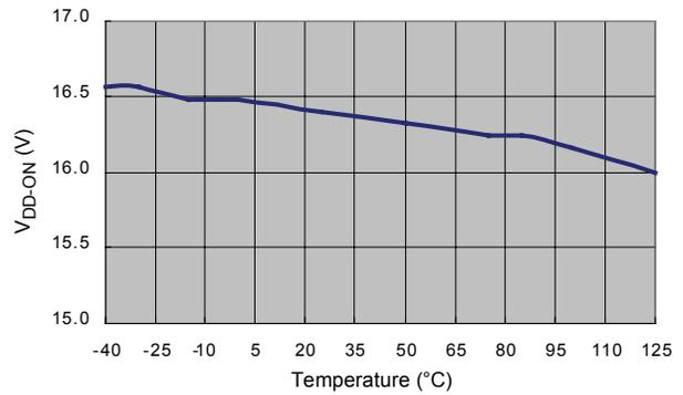
**Figure 9. Start Threshold Voltage ( $V_{DD-ON}$ ) vs. Temperature**
