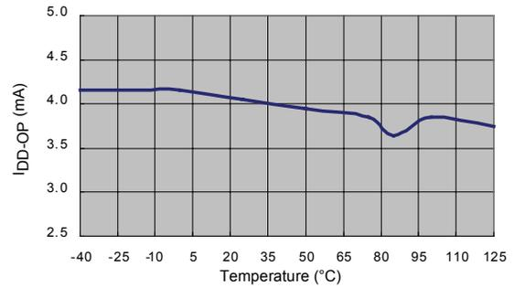
**Figure 7. Operating Supply Current ( $I_{DD-OP}$ ) vs. Temperature**
