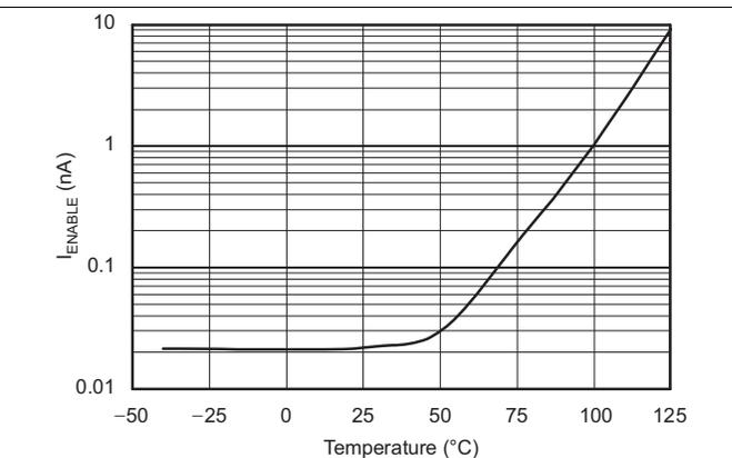
Figure 24.  $I_{ENABLE}$  vs Temperature
