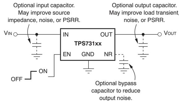
Figure 31. Typical Application Circuit for Fixed-Voltage Versions
