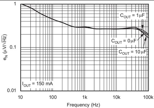
Figure 15. Noise Spectral Density  $C_{NR} = 0\text{ }\mu\text{F}$
