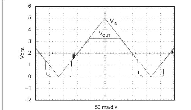
Figure 23. TPS73133 Power Up and Power Down
