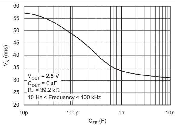
Figure 25. TPS73101 RMS Noise Voltage vs  $C_{FB}$
