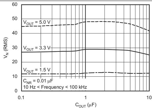
Figure 17. RMS Noise Voltage vs  $C_{OUT}$
