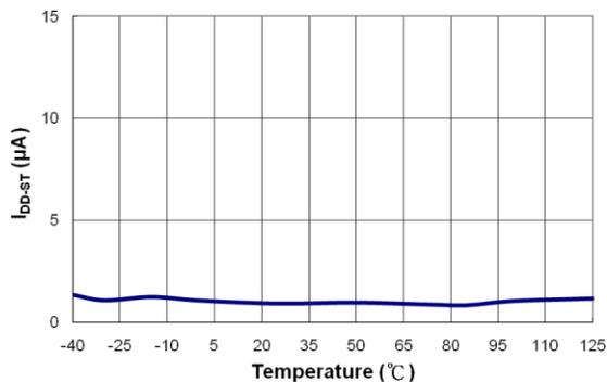
Figure 8. Startup Current ( $I_{DD-ST}$ ) vs. Temperature
