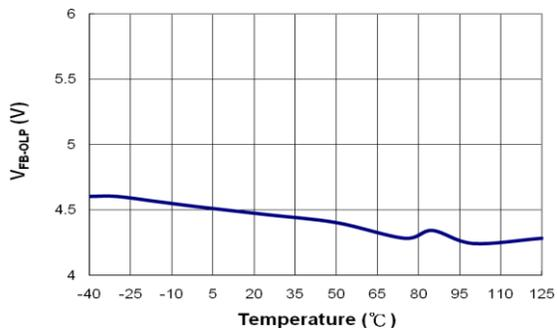
Figure 16. FB Open-Loop Trigger Level (V<sub>FB-OLP</sub>) vs. Temperature
