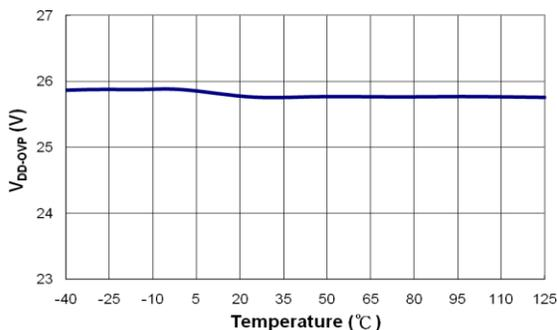
Figure 19. V<sub>DD</sub> Over-Voltage Protection (V<sub>DD-OVP</sub>) vs. Temperature
