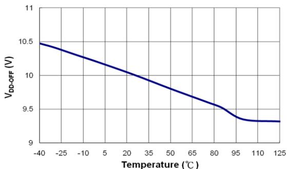
Figure 11. Minimum Operating Voltage ( $V_{DD-OFF}$ ) vs. Temperature
