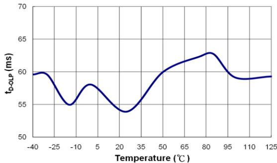
Figure 17. Delay Time of FB Pin Open-Loop Protection (t<sub>D-OLP</sub>) vs. Temperature
