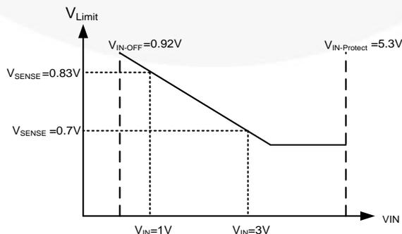
**Figure 6.  $V_{IN}$  vs.  $V_{SENSE}$**
