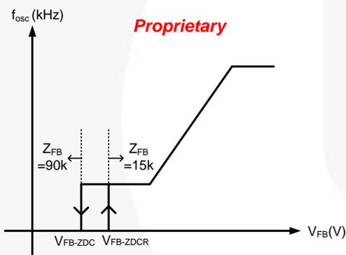
Figure 22. Z<sub>FB</sub>-Switching Activating Range
