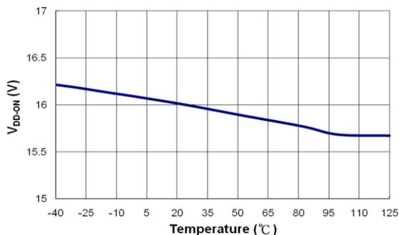
Figure 10. Start Threshold Voltage ( $V_{DD-ON}$ ) vs. Temperature
