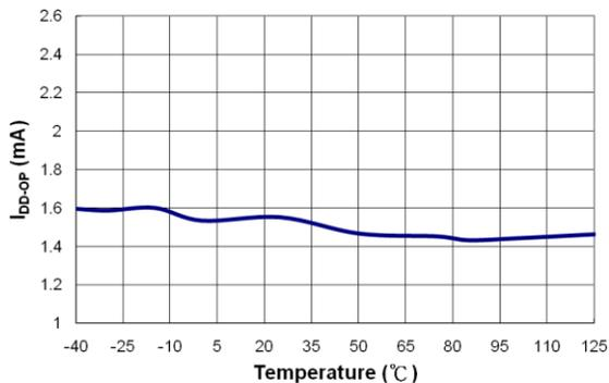
Figure 9. Operation Supply Current ( $I_{DD-OP}$ ) vs. Temperature
