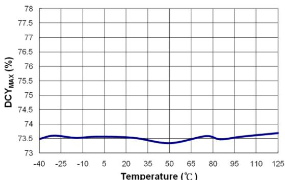
Figure 15. Maximum Duty Cycle ( $DCY_{MAX}$ ) vs. Temperature
