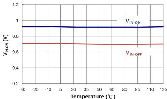
Figure 18. PWM Turn-Off Threshold Voltage (V<sub>IN-OFF</sub> & V<sub>IN-ON</sub>) vs. Temperature
