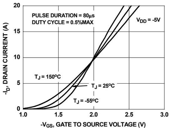
**Figure 5. Transfer Characteristics**
