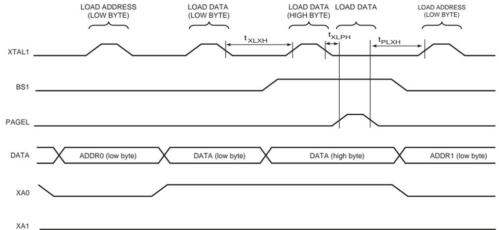
Note: 1. The timing requirements shown in Figure 102 (i.e.,  $t_{DVXH}$ ,  $t_{XHXL}$ , and  $t_{XLDX}$ ) also apply to loading operation.
