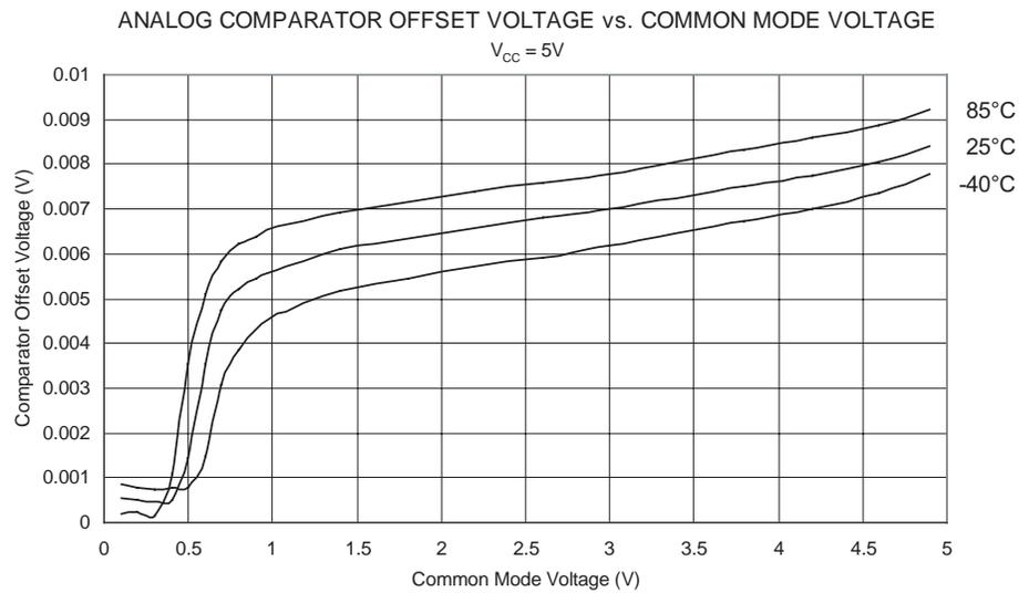
**Figure 165.** Analog Comparator Offset Voltage vs. Common Mode Voltage ( $V_{CC} = 2.7V$ )
