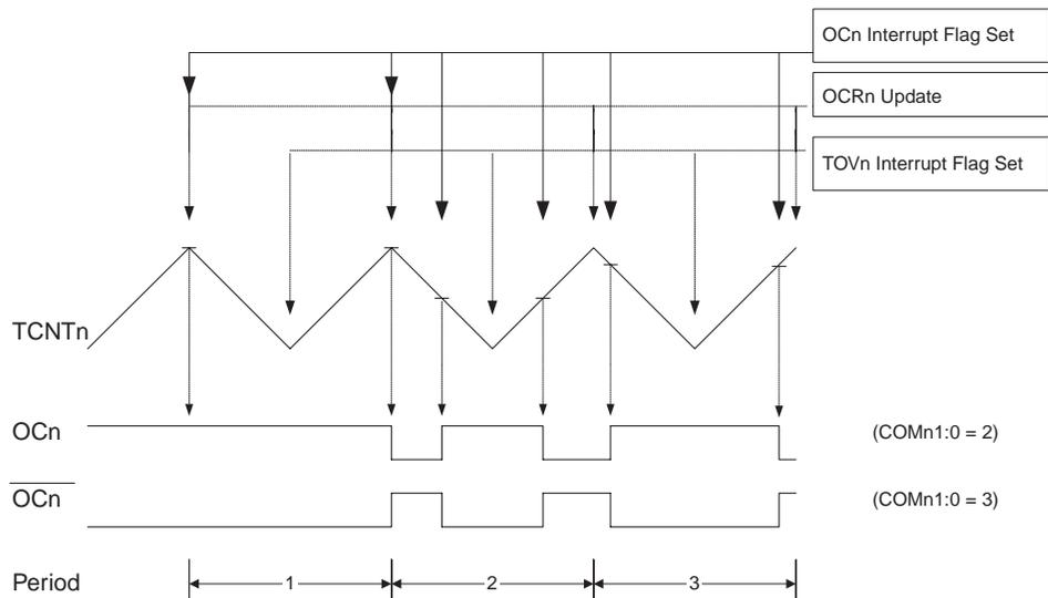
The Timer/Counter Overflow Flag (TOV2) is set each time the counter reaches BOTTOM. The Interrupt Flag can be used to generate an interrupt each time the counter reaches the BOTTOM value.
