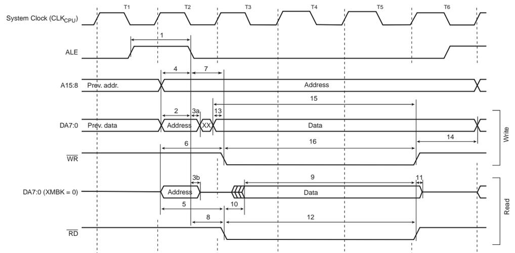
**Figure 121. External Memory Timing (SRWn1 = 1, SRWn0 = 1)<sup>(1)</sup>**
