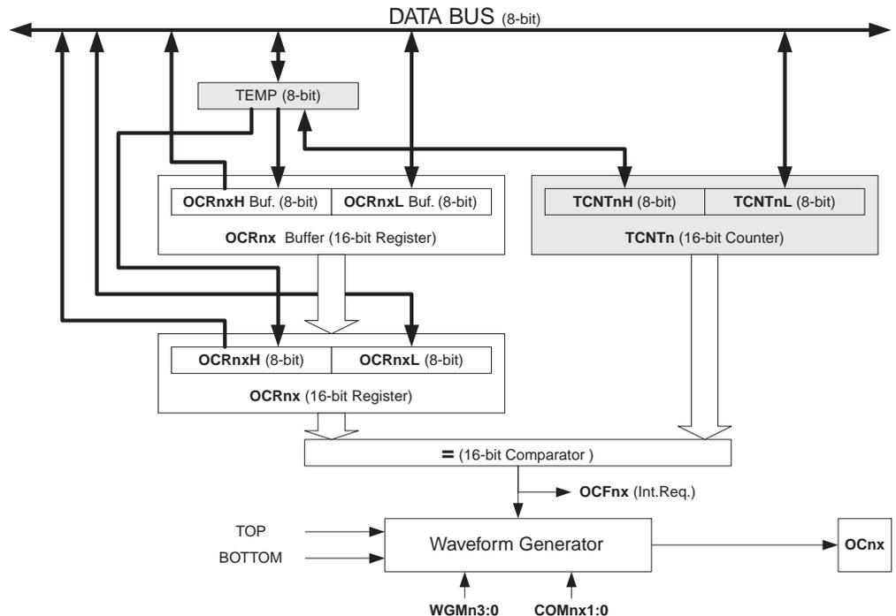
The OCRnx Register is double buffered when using any of the twelve *Pulse Width Modulation* (PWM) modes. For the normal and *Clear Timer on Compare* (CTC) modes of operation, the double buffering is disabled. The double buffering synchronizes the update of the OCRnx Compare Register to either TOP or BOTTOM of the counting
