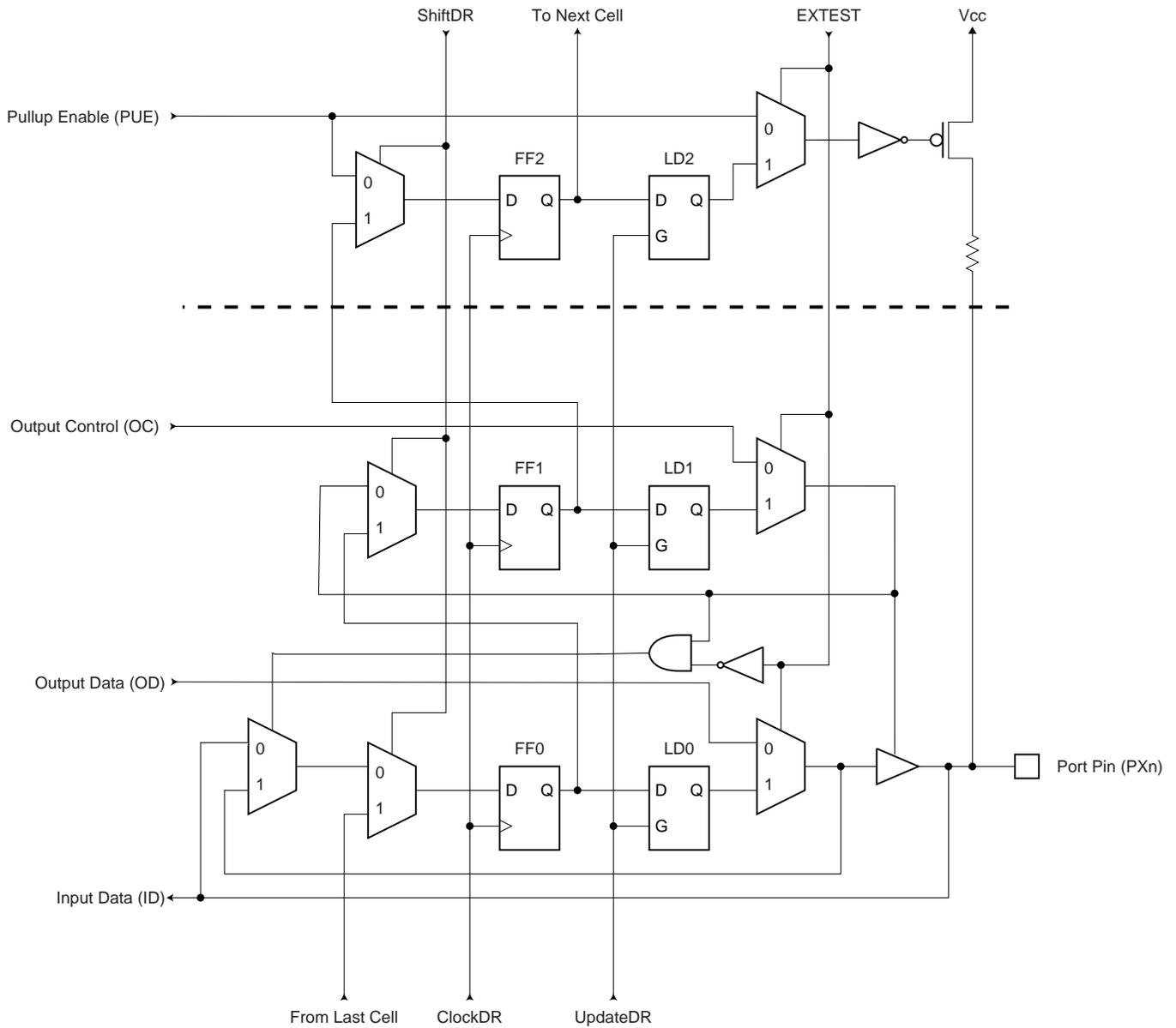
**Figure 88.** General Port Pin Schematic Diagram
