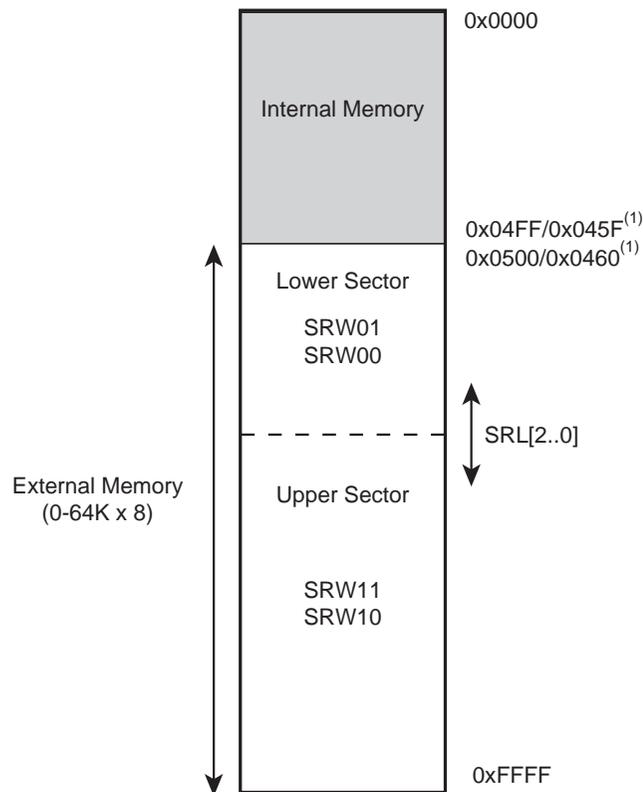
Note: 1. Address depends on the ATmega161 compatibility Fuse. See “SRAM Data Memory” on page 16 and Figure 9 on page 17 for details.
