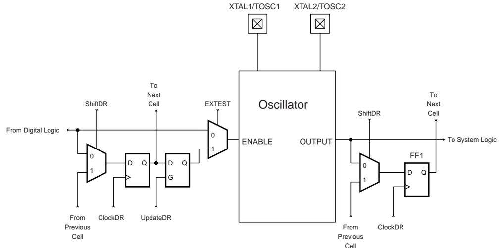
Table 86 summarizes the scan registers for the external clock pin XTAL1, oscillators with XTAL1/XTAL2 connections as well as 32 kHz Timer Oscillator.
