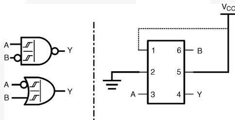
Figure 6. 2-Input NAND with Inverted B Input
