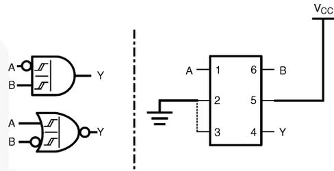
**Figure 10. 2-Input AND with Inverted A Input**
