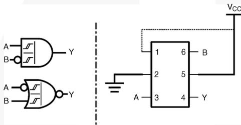
**Figure 11. 2-Input AND with Inverted B Input**
