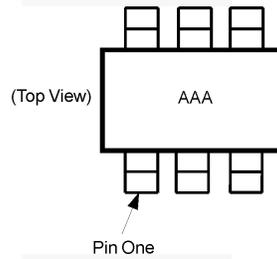
Figure 3. Pin 1 Orientation
