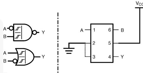
Figure 5. 2-Input NAND with Inverted A Input
