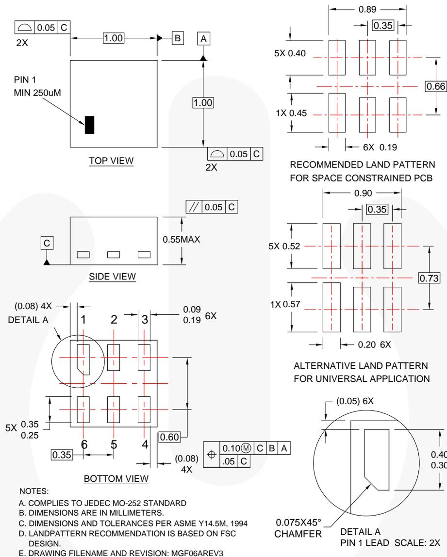
**Figure 19. 6-Lead, MicroPak2™, 1x1mm Body, .35mm Pitch**
