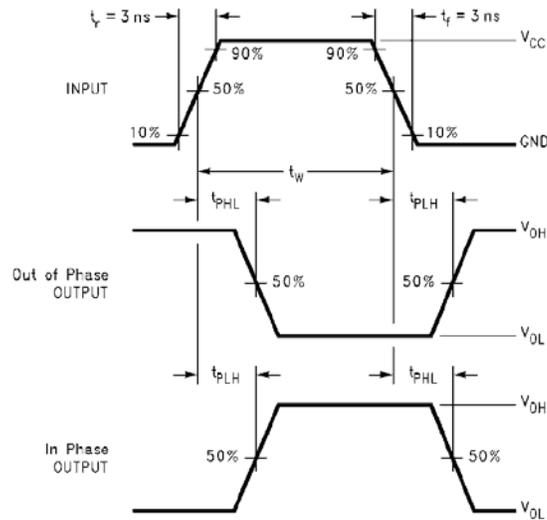
**Figure 16. AC Waveforms**
