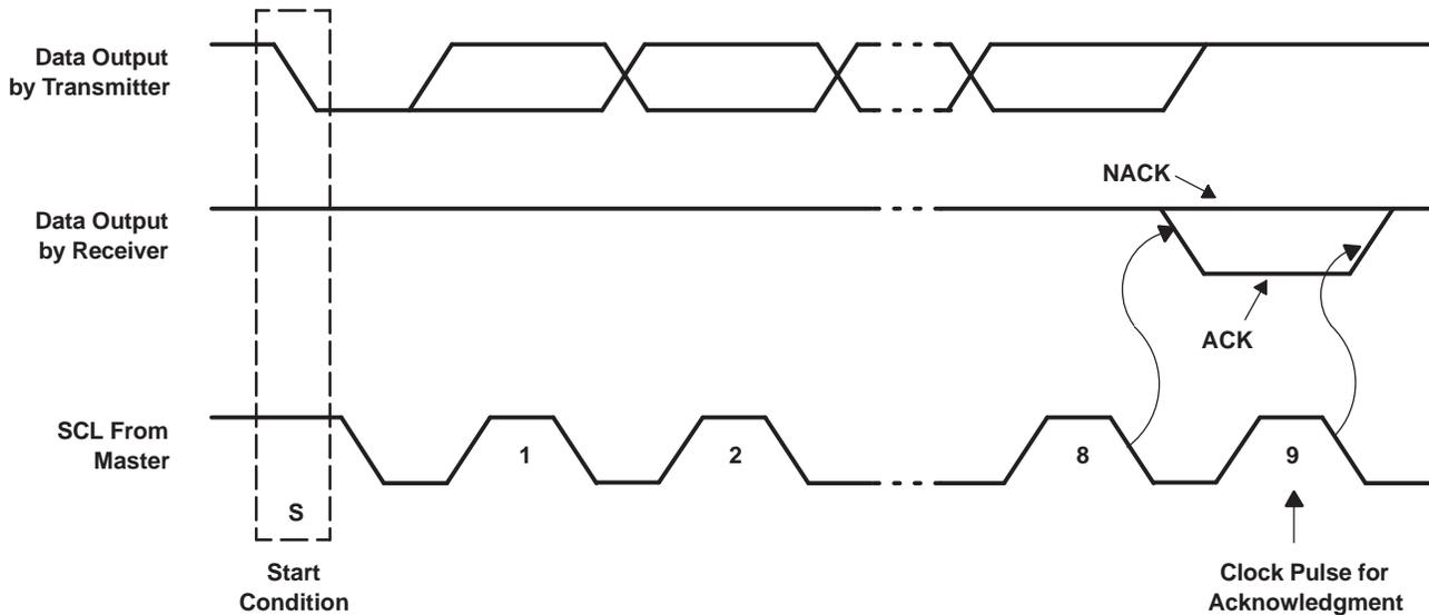
Figure 21. Acknowledgment On The I<sup>2</sup>C Bus
