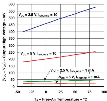
Figure 11. Output High Voltage vs Temperature (P7-P1)
