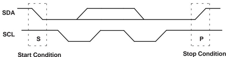
**Figure 19. Definition Of Start And Stop Conditions**
