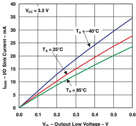
Figure 5. I/O Sink Current vs Output Low Voltage
