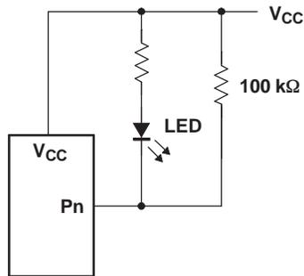
**Figure 29. High-Value Resistor In Parallel With The Led**
