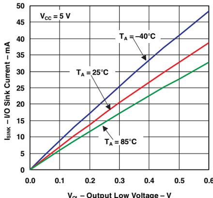
Figure 6. I/O Sink Current vs Output Low Voltage
