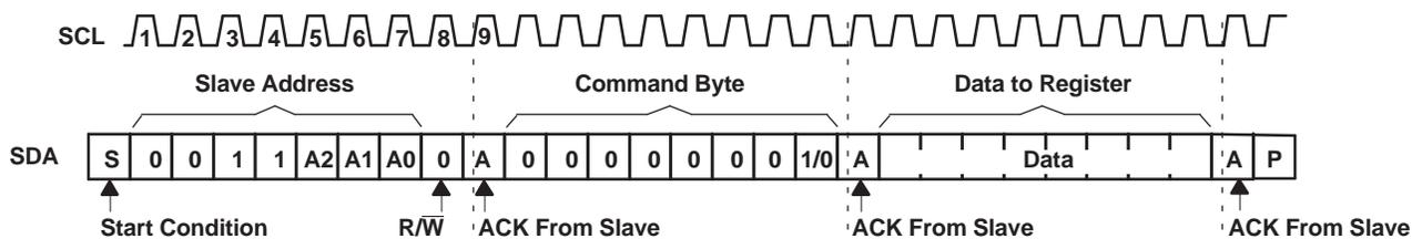
Figure 25. Write To Configuration Or Polarity Inversion Registers
