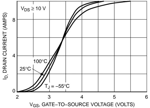
Figure 2. Transfer Characteristics
