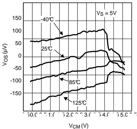
Figure 11. Input Offset Voltage vs. Input Common Mode
