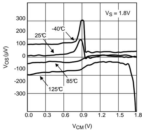
Figure 9. Input Offset Voltage vs. Input Common Mode
