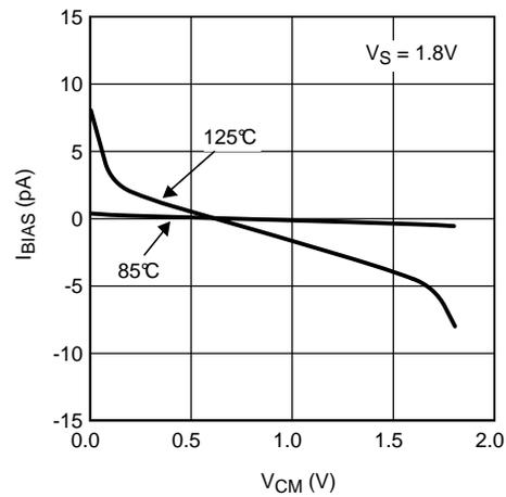
Figure 34. Input Bias Current vs. Common Mode Voltage
