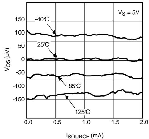
Figure 22. Input Offset Voltage vs. Sinking Current
