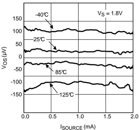
Figure 17. Input Offset Voltage vs. Sourcing Current
