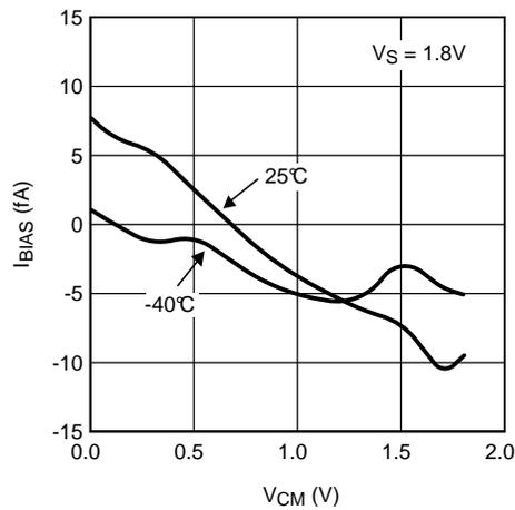
Figure 33. Input Bias Current vs. Common Mode Voltage
