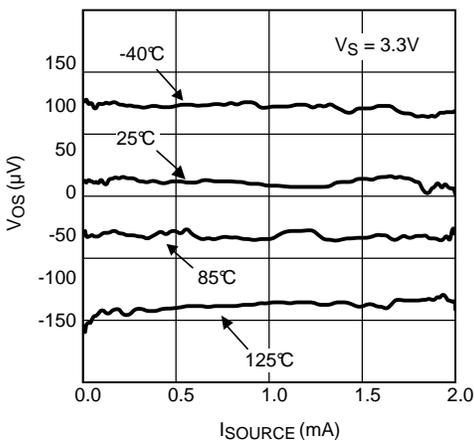
Figure 18. Input Offset Voltage vs. Sourcing Current
