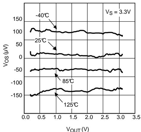
Figure 15. Input Offset Voltage vs. Output Voltage
