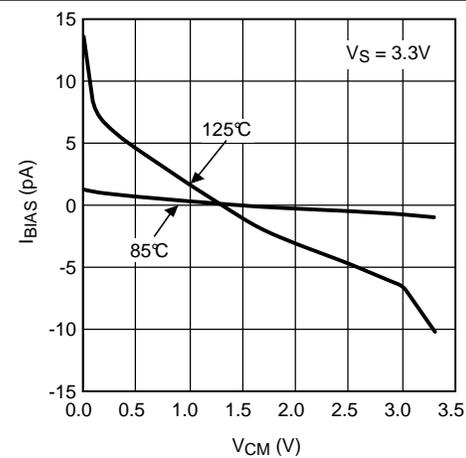
Figure 36. Input Bias Current vs. Common Mode Voltage
