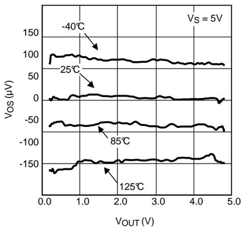
Figure 16. Input Offset Voltage vs. Output Voltage
