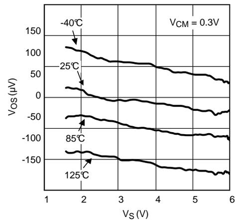
Figure 12. Input Offset Voltage vs. Supply Voltage
