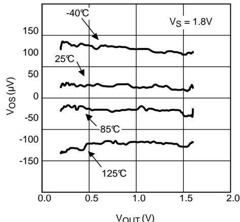
Figure 14. Input Offset Voltage vs. Output Voltage
