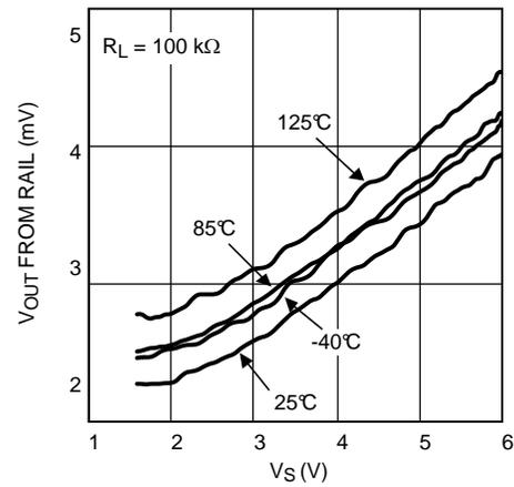
Figure 32. Output Swing Low vs. Supply Voltage
