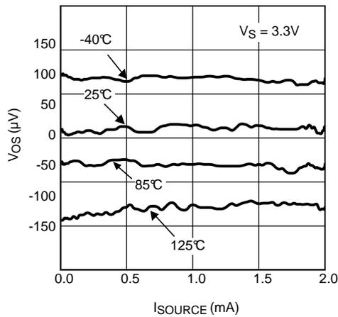
Figure 21. Input Offset Voltage vs. Sinking Current
