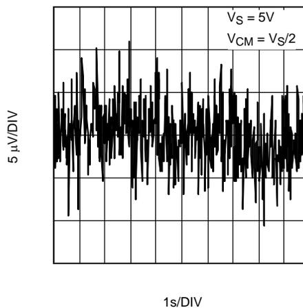
Figure 54. 0.1 to 10 Hz Time Domain Voltage Noise
