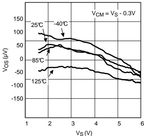
Figure 13. Input Offset Voltage vs. Supply Voltage
