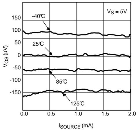
Figure 19. Input Offset Voltage vs. Sourcing Current
