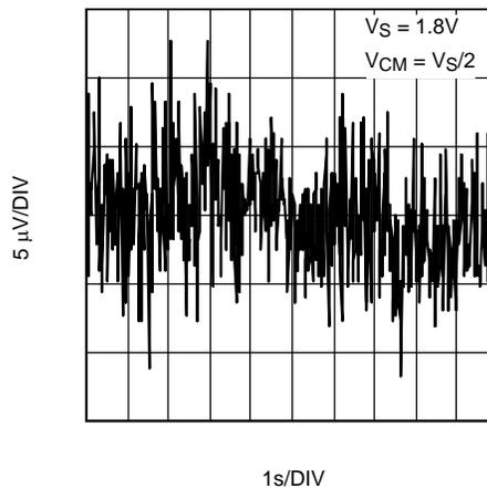
Figure 52. 0.1 to 10 Hz Time Domain Voltage Noise
