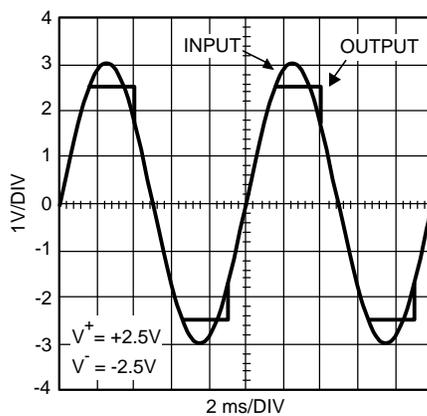
Figure 59. Overload Recovery Waveform
