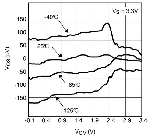
Figure 10. Input Offset Voltage vs. Input Common Mode
