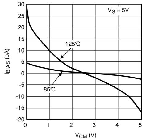
Figure 38. Input Bias Current vs. Common Mode Voltage
