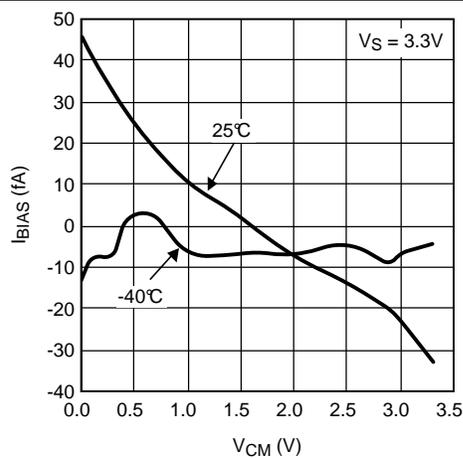
Figure 35. Input Bias Current vs. Common Mode Voltage
