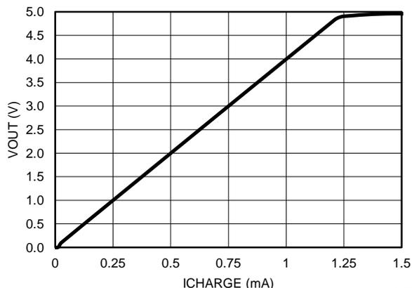
Figure 69. Calculated High-Side Current Sense Circuit Output
