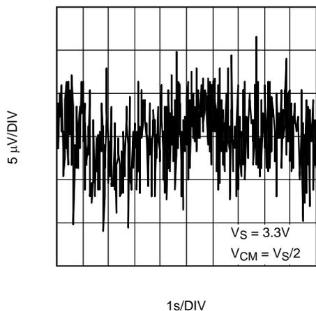
Figure 53. 0.1 to 10 Hz Time Domain Voltage Noise
