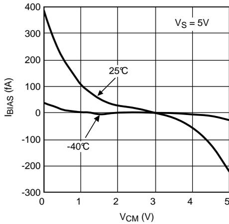
Figure 37. Input Bias Current vs. Common Mode Voltage
