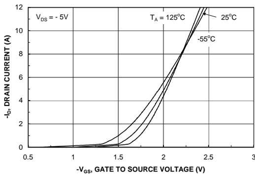
Figure 5. Transfer Characteristics.
