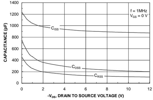
Figure 8. Capacitance Characteristics.
