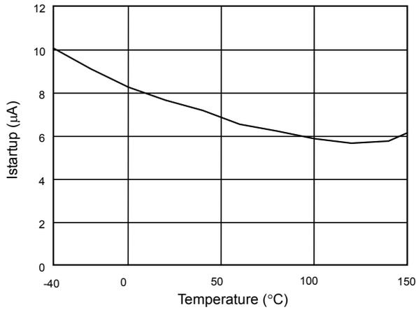
Fig. 1 Startup Current (I<sub>startup</sub>) vs. Temperature
