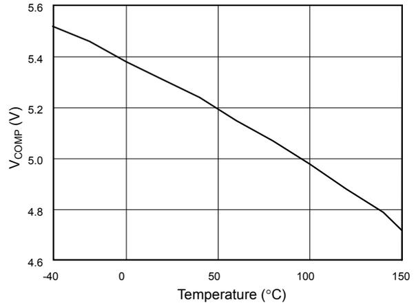
Fig. 2 V<sub>COMP</sub> open loop voltage v.s. Temperature
