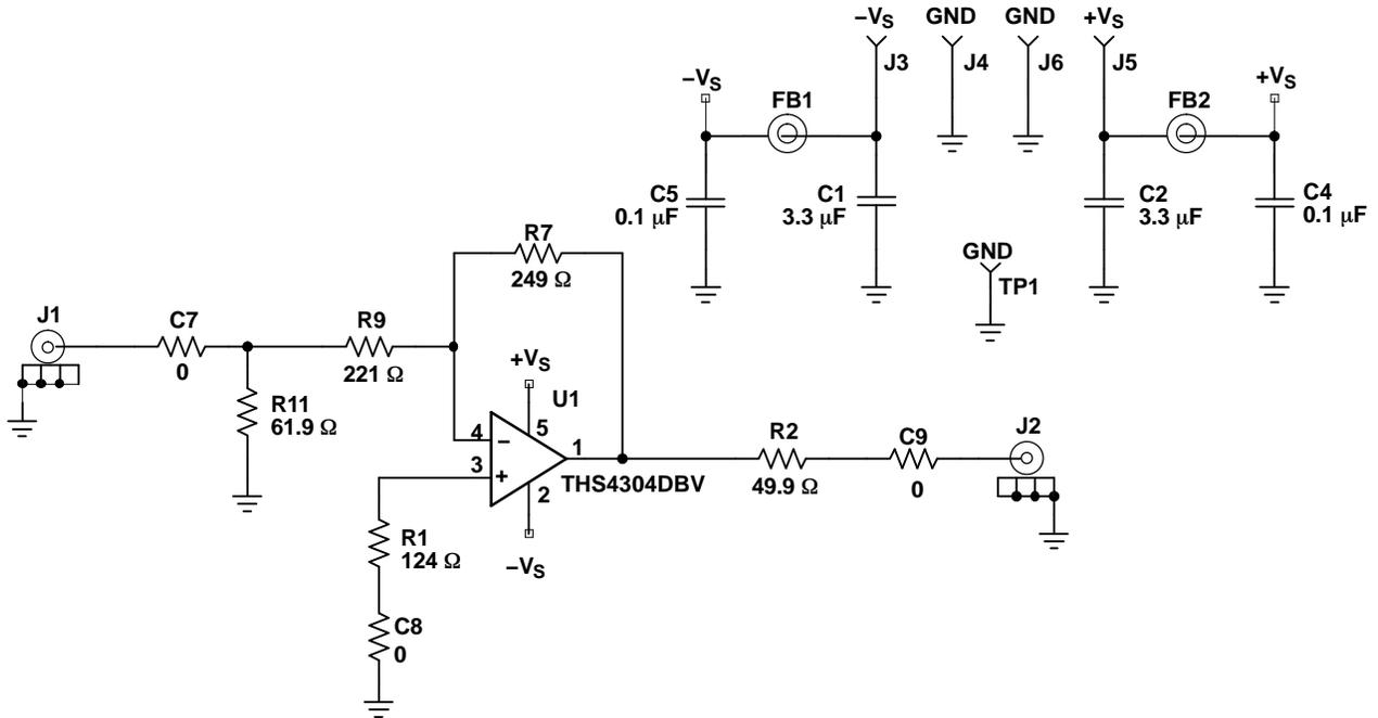
**Figure 53. Inverting Gain with Split Power Supply**
