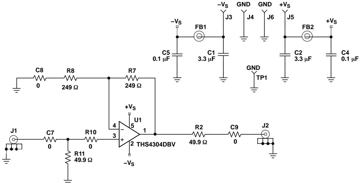
**Figure 52. Non-Inverting Gain with Split Power Supply**
