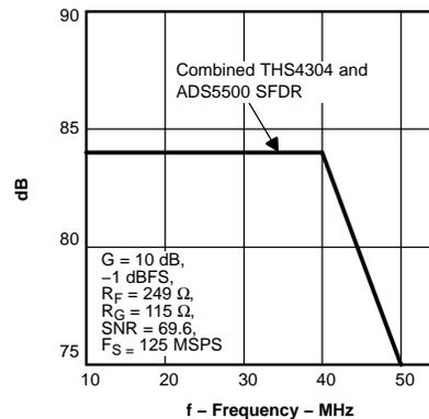
Figure 56. SFDR Performance versus Frequency – THS4304 Driving ADS5500
