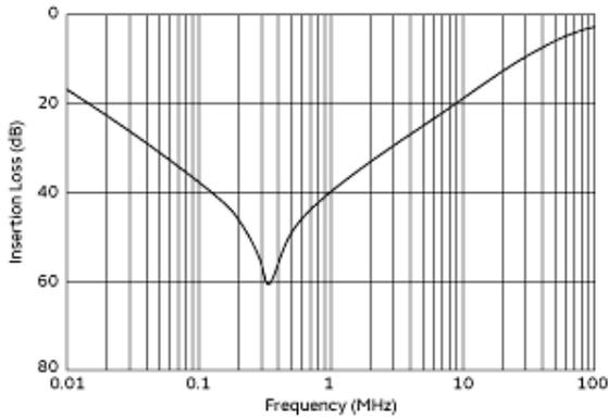
Common Mode Insertion Loss (Typ.)
