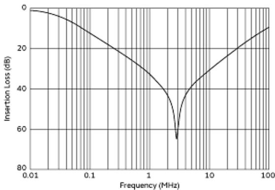
Differential Mode Insertion Loss (Typ.)
