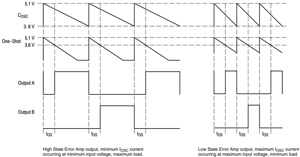
Figure 15. Timing Diagram
