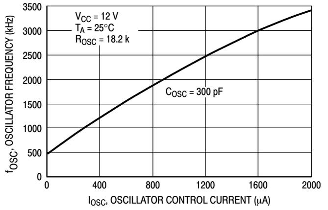
**Figure 3. Oscillator Frequency versus Oscillator Control Current**
