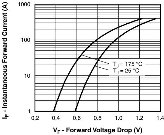
Fig. 1 - Typical Forward Voltage Drop Characteristics (Per Diode)
