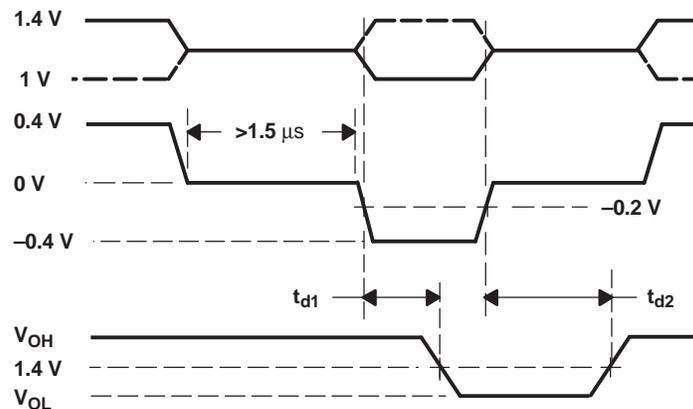
**Figure 6. Waveforms for Failsafe Activate and Deactivate**
