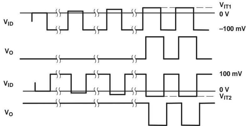
NOTE: Input signal of 3 Mpps, duration of 167 ns, and transition time of <1 ns.
